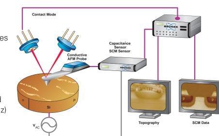
measurements to be taken more reliably and on a much wider range of samples, as well as allowing for the direct correlation of electrical data with nanomechanical information from PeakForce QNM<sup>™</sup> measurements. Applications range from studies of
