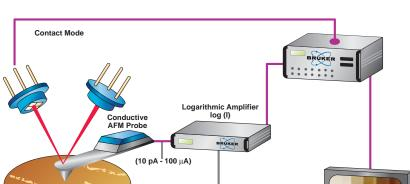
Scanning Capacitance Microscopy (SCM) can be used on flat, well-prepared semiconductor surfaces to map the relative changes of majority carrier concentrations. SCM operates in contact mode by forming a metal-insulator-semiconductor capacitor between the tip and the sample. This capacitor is measured using an ultrahigh-frequency (1 GHz) detector as it is varied with an applied AC + DC bias. The AC (~90 kHz) + DC bias is set to create
