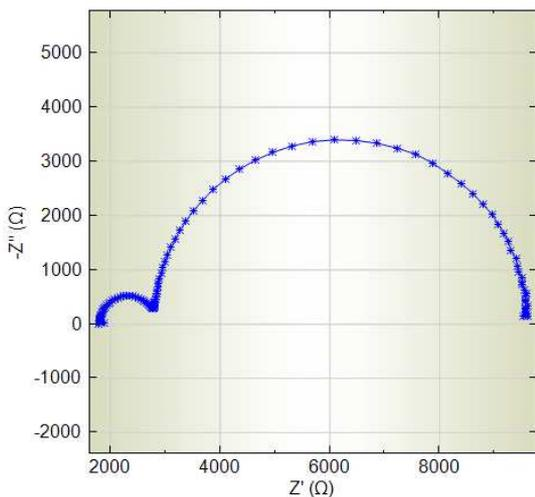
An equivalent circuit that consists of two RC time constants can model this spectrum. The two RC time constants can be produced by combining the resistances and capacitances in three different ways resulting in three equivalent circuits shown in the following figure. All three circuits when fitted to
