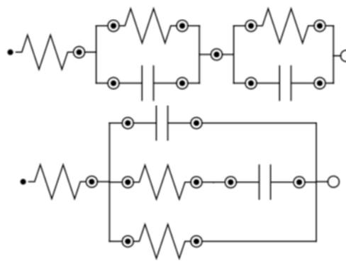
The three equivalent circuits shown above are mathematically identical.
