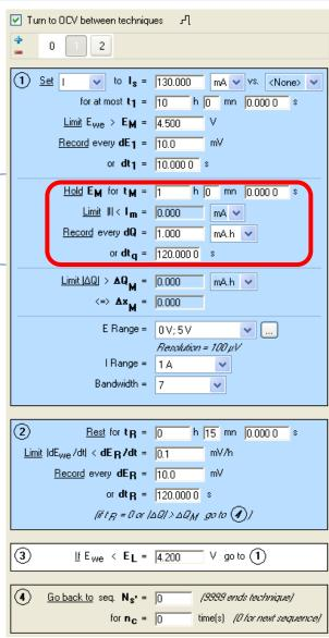
• This block allows the user to complete the charge/discharge in potentiostatic mode (in the first block the charge/discharge was performed in galvanostatic mode).
