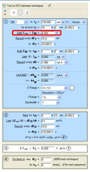
Define the **max** voltage until which the **charge** has to be performed.
