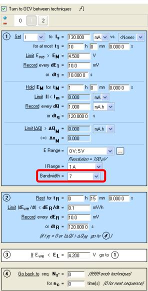
This parameter defines the stability/speed (regulation loop) of the instrument. As battery have a slow response, a slow bandwidth will be appropriate. Bandwidth of 5 for VMP3 family and 7 for SP-300 family is often appropriate. (See manuals and application note for more information bandwidth).
