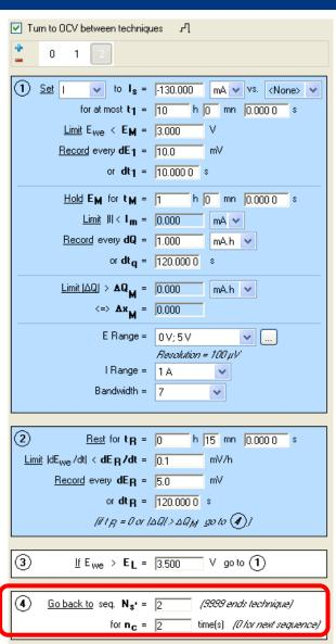
This allows the user to loop on a sequence of charge/discharge within the GCPL technique. The user defines at which sequence the protocol will go back and for how many times.
