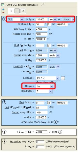
• Defines the applied current. It is positive for charge and negative for discharge. If the capacity of the battery is defined in the "Cell characteristics", the user may select a rate instead of a current.
