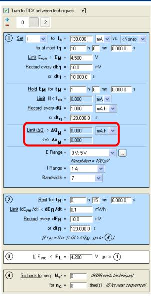
This is the limit on the total charge exchanged during the sequence. This limit can also be defined with the intercalation coefficient.
