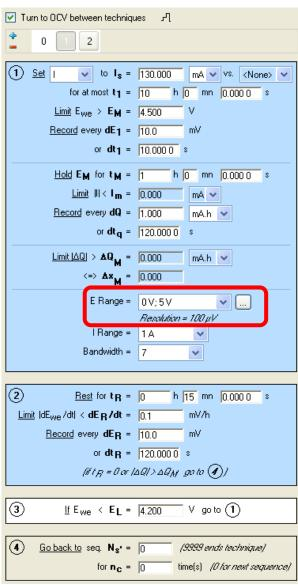
The Erange has to be wide enough to be in the range of the operating voltage of the battery but narrow enough to get an optimized resolution in the voltage measurement/control.
