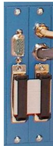
Fig. 53: Standard channel connected to a "p" low current board.
