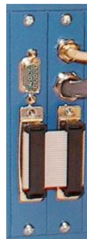
Fig. 9: Standard channel connected to a 'p' low current board.
