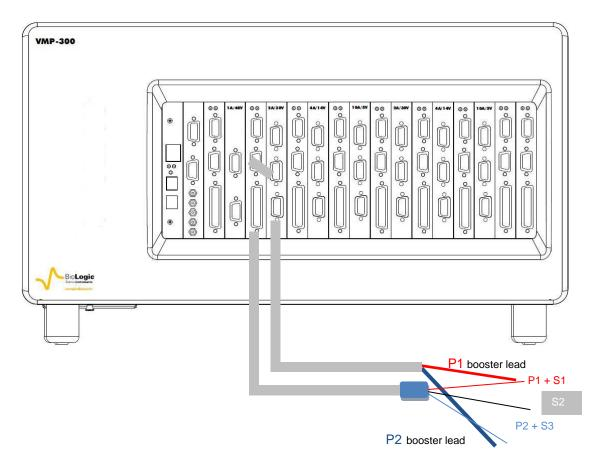
Fig. 63: Channel board connection to the cell with one 2A/30V booster
