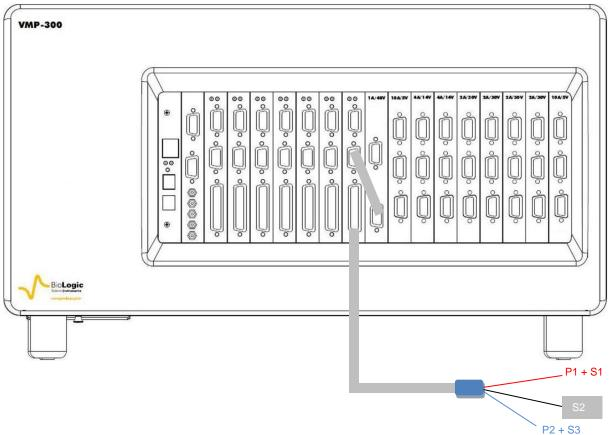
Fig. 62: Channel board connection to the cell with the 1A/48V booster.
