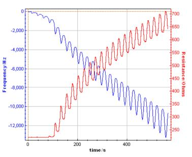
Fig. 76: Frequency and resistance variations recorded from the analog inputs for an instrument coupled with a SEIKO EG&G QCM 922.
