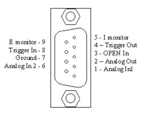
Fig. 65: Structure of the DB9 connector.
