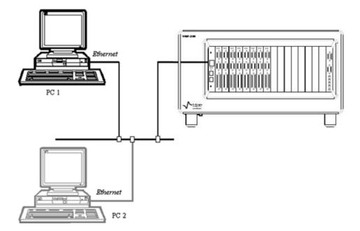
Fig. 26: Ethernet cable for network connection (1 INSTRUMENT, several PCs).
