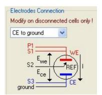
Fig. 58: CE to Ground connection mode.
