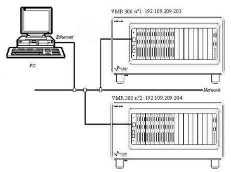
Fig. 27: Network connection: one PC to several instruments.
