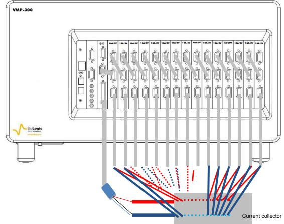
Fig. 64: Channel board connection to the cell with fifteen boosters.
