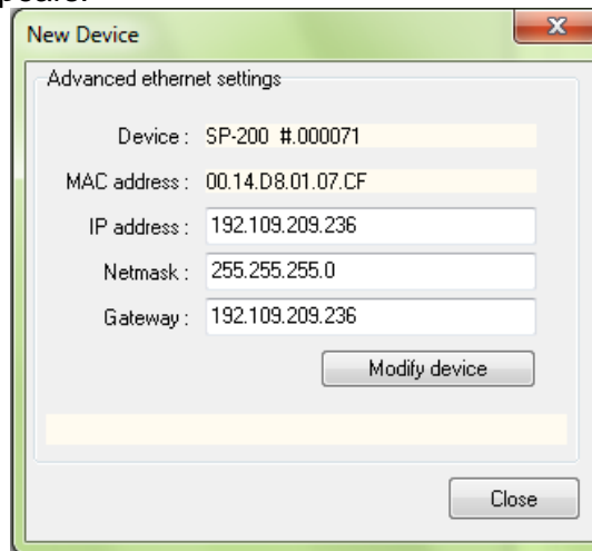
Fig. 43: “Advanced Ethernet settings” of the “New Device” window used to change the instrument IP Address.
