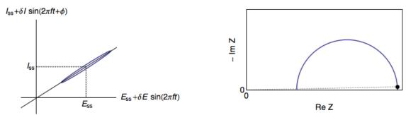
Increasing the frequency  $\rightarrow$  moving away from the steady-state response
