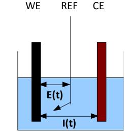
A three-electrode set-up is required.
