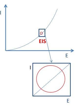
EIS is a local measurement at one point on the steady-state curve.
