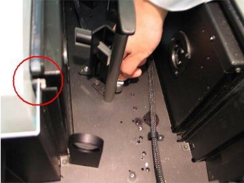
**Figure 23.** Place the front lock down pin into position.
