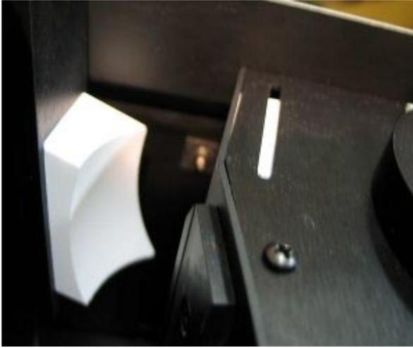
**Figure 20.** Install the specular port plug.
