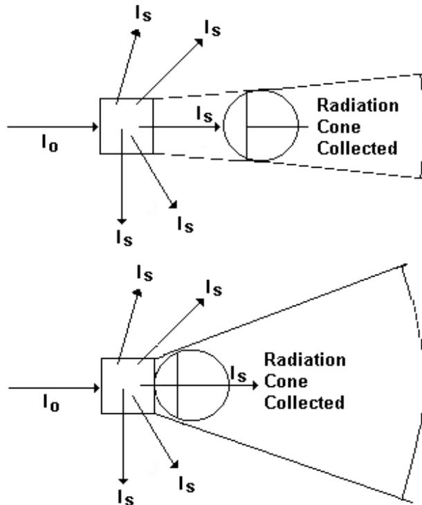
**Figure 4:** Collection of scattered light by an integrating sphere.  $I_o$  = incident light,  $I_s$  = scattered light.
