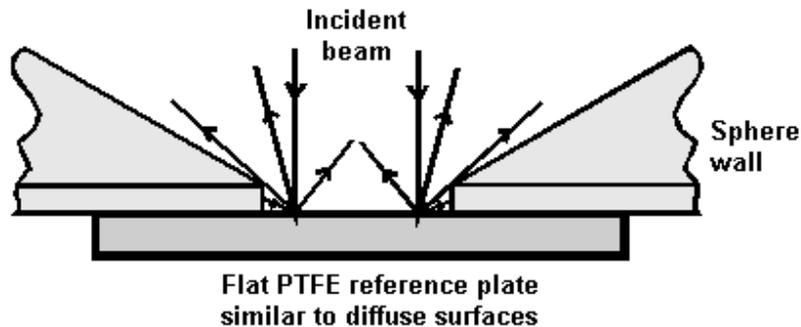
*Figure 7: Highly diffuse samples are measured against a flat PTFE reference plate*
