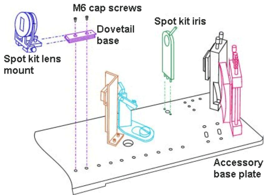
**Figure 35:** *Installing the small spot kit.*
