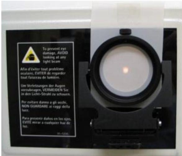
**Figure 37.** The beam from the small spot kit with the iris partially open.
