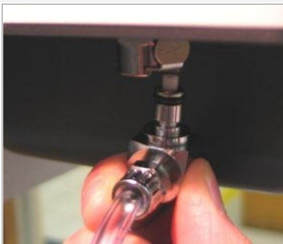
**Figure 54.** Attach the connector on the hose to the connector on the under side of the integrating sphere.
