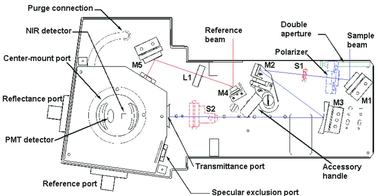
**Figure 9:** A schematic view of the external DRA.
