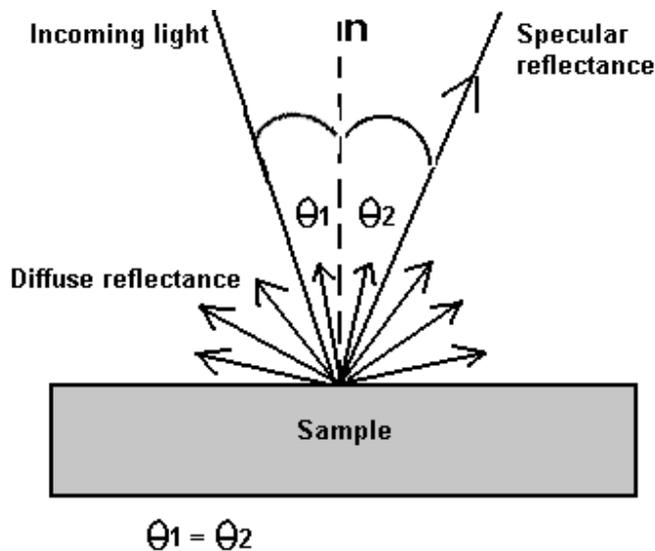
**Figure 3:** The two components of reflection: specular and diffuse reflection.  $n$  represents the surface normal, an imaginary line at  $90^\circ$  to the sample surface.
