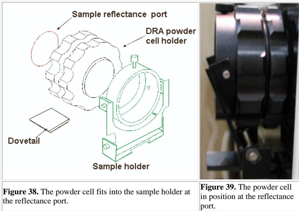
The design of the PCH-150 sample holder does not facilitate an accurate means of loading a powdered sample to an accurate packing density. An approximate packing density and reflectance measurement can be obtained using the following procedures. Prior to loading, the sample should be ground to the desired particle size.
