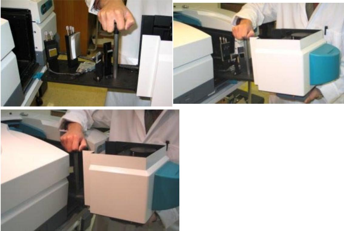
9. Take care to align the metal edges of the DRA with the guide tabs on the edge of the instrument sample compartment. This will correctly align and engage the rear lockdown pins into the the sample compartment floor. The following two photos illustrate how to line up the tabs, note inparticular the red circle indicating where the tabs should sit.
