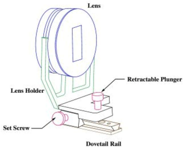
*Figure 34: The small spot kit lens holder, rail and lens.*
