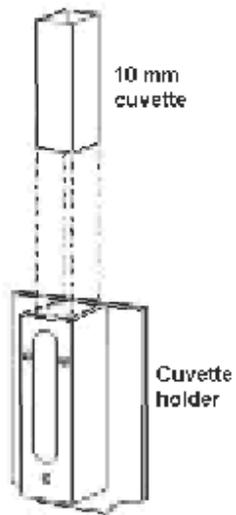
*Figure 29: The cuvette holder*
