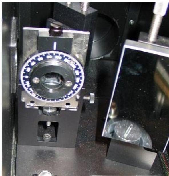
**Figure 45. The polarizer attachment in the DRA.**
