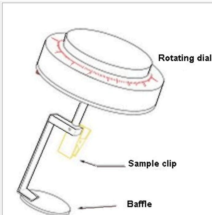
**Figure 31:** The clip style variable angle sample holder.
