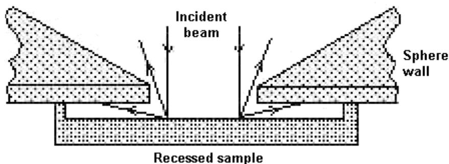
**Figure 5:** Some of the wide-angle scatter is lost when there is a space between the sample and the sphere wall
