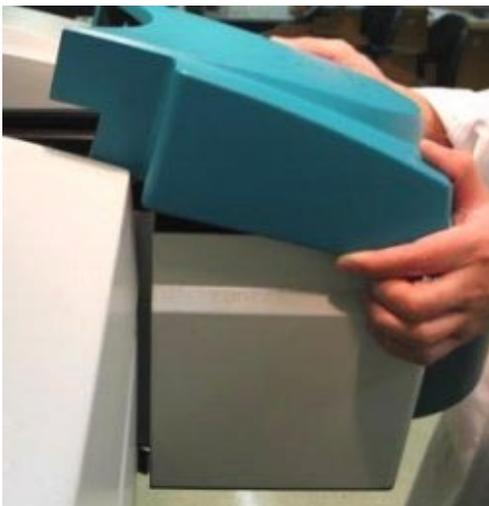
**Figure 46.** Removing the accessory cover.
