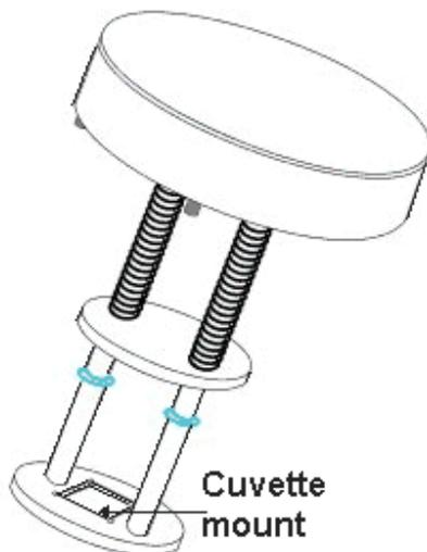
**Figure 33:** *The cuvette variable sample holder.*
