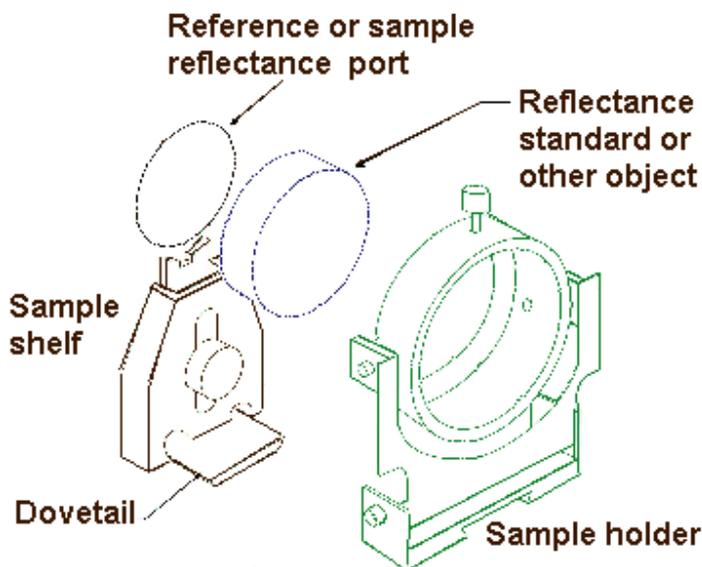
**Figure 24.** The sample holder fits onto the dovetail at either the reference or reflectance port.
