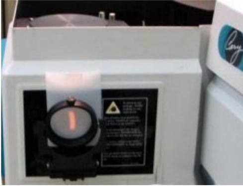
**Figure 27.** Checking the beam at the reference port.
