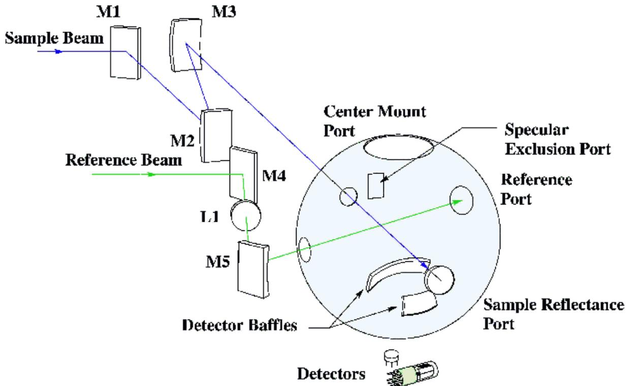
*Figure 10: The optical design of the external DRA.*
