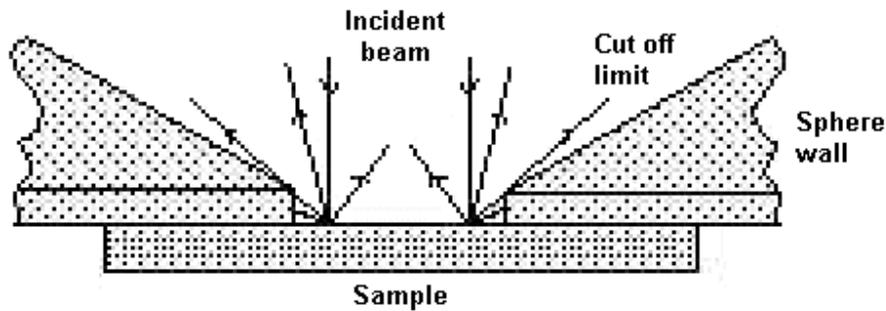
*Figure 6: Some of the wide-angle reflection is intercepted by the sphere wall*
