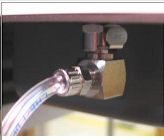
**Figure 55.** The connectors snap together.
