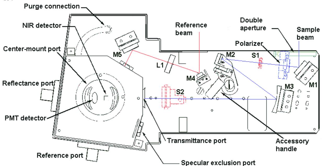
**Figure 19:** The Varian 900, 1800, 2500 Diffuse Reflectance accessory with the optics cover removed. The large reference plate is clamped over the sample port at the centre of the sphere cap.
