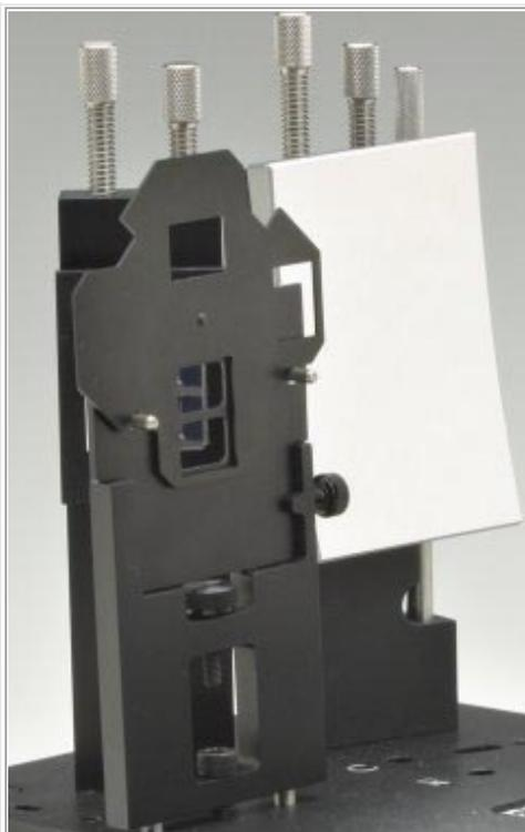
**Figure 43.** The double aperture attachment on the polarizer mount.
