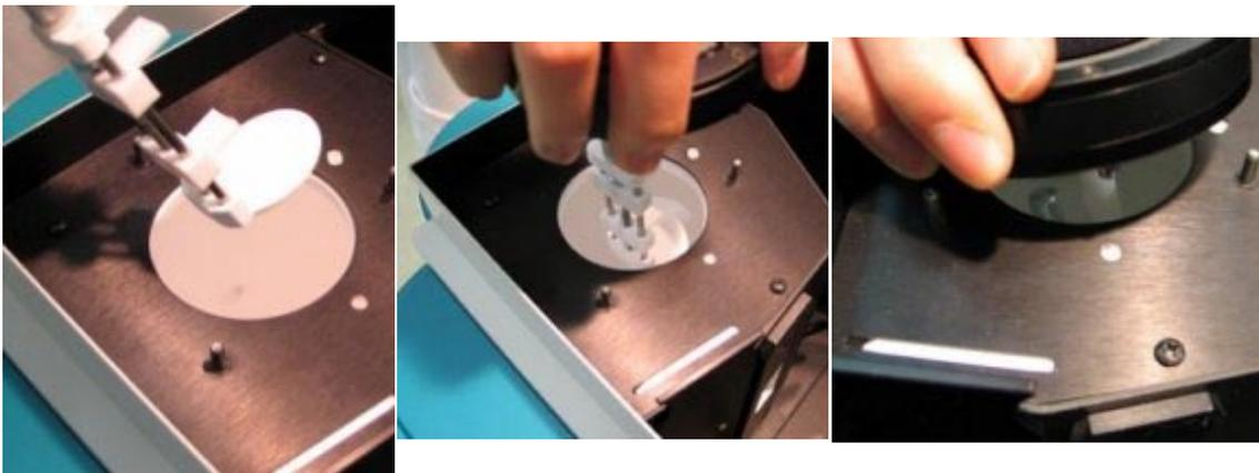
**Figure 30.** Lower the centre mount through the opening in the sphere, use the locating holes in the top of the sphere to secure the centre mount.
