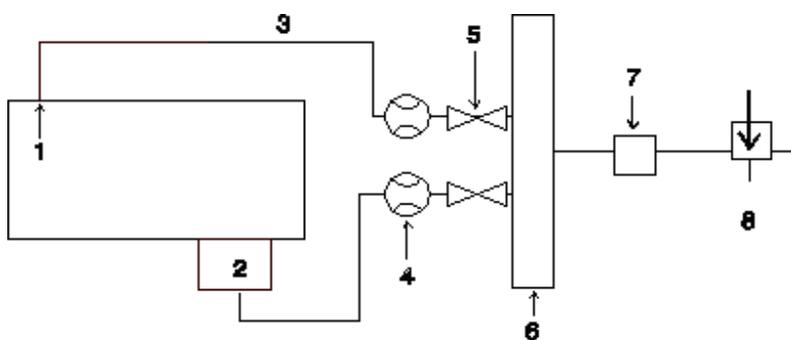
Figure 53. The position of flowmeters when purging with nitrogen:
