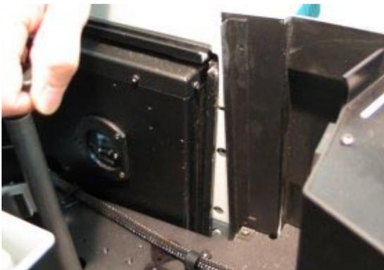
**Figure 22.** Align the tabs on the DRA with those on the instrument sample compartment.
