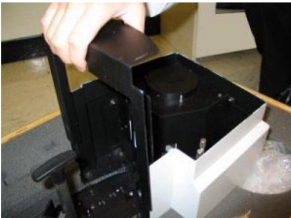
**Figure 17.** Removing the light seal.
