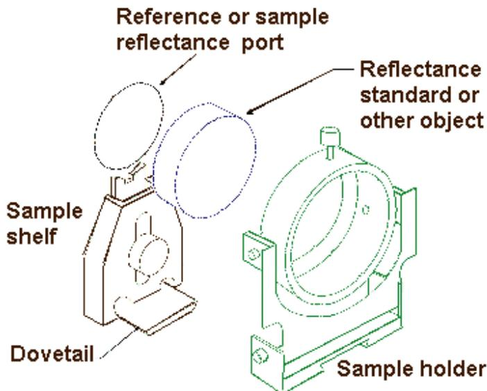
**Figure 48.** The sample is mounted at the reflectance or reference port using the sample holder.
