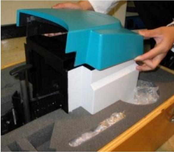
**Figure 16.** Removing the accessory cover.
