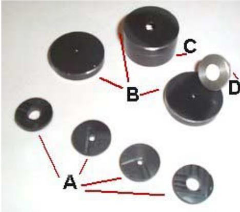
**Figure 21.** The Small Sample mount. "A" sample mounts, "B" apertures, "C" sample cup and "D" PTFE standard.
