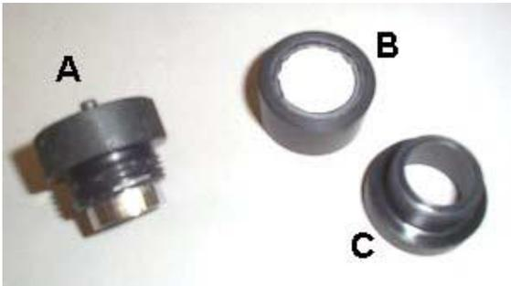
*Figure 19. The powder cell. A = lid, B = sample cup, C = funnel.*
