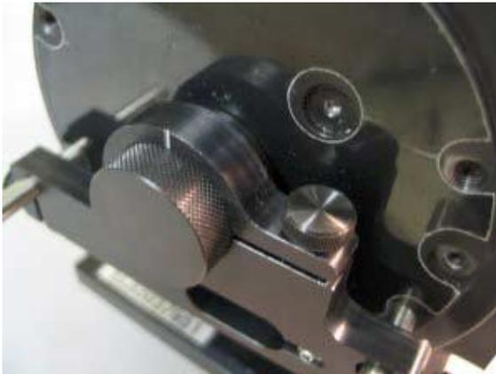
**Figure 21.** The powder cell fitted into the small sample holder, note that the textured edge of the powder cell sits flush with the edge of the small sample holder. The screw to the right of the powder cell is used to secure the powder cell.
