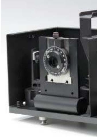
**Figure 26.** The polarizer installed on the polarizer mount.
