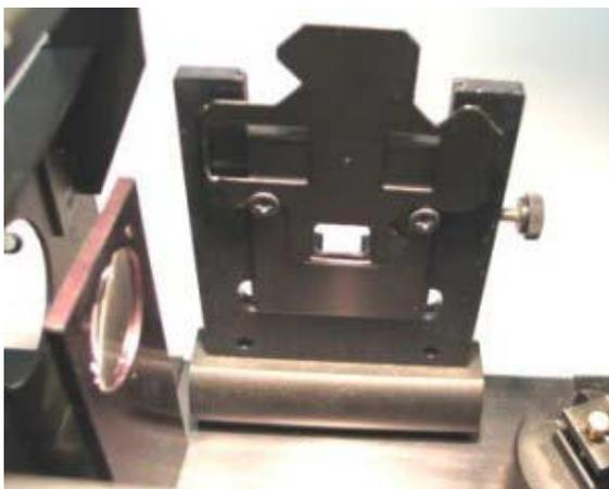
**Figure 29.** The mask fits onto the double aperture base. This figure shows only one aperture is open.
