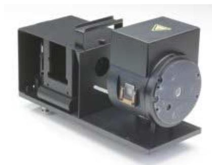
**Figure 10.** The internal DRA. Note the clips on the left hand side of the accessory. These are for attaching metal screens during [reference beam attenuation](#).
