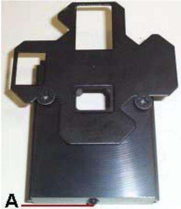
**Figure 27.** The Double Aperture attachment. A indicates the locating pin at the bottom of the attachment.
