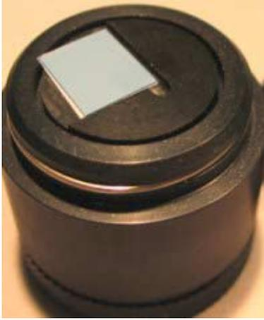
**Figure 23.** The mask and sample are placed on the sample cup.
