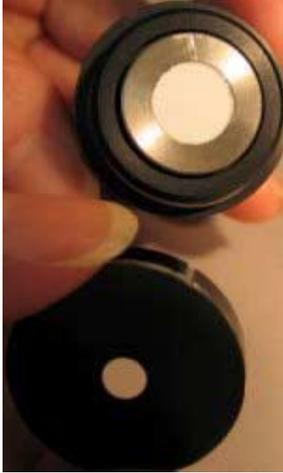
**Figure 25.** The PTFE standard fits into the sample cup.
