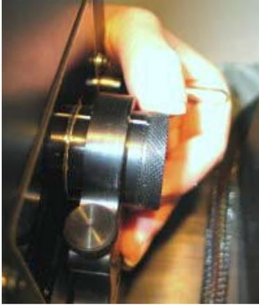
**Figure 24.** The small sample mount fits into the small sample holder. Note that in this picture the small sample holder and small sample mount are in the correct position for performing transmission measurements.
