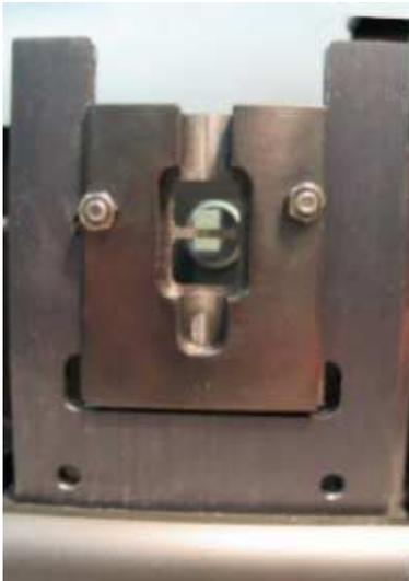
**Figure 28.** Install the double aperture base onto the polarizer mount.
