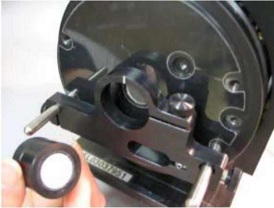
**Figure 20.** Insert the powder cell into the small sample holder.
