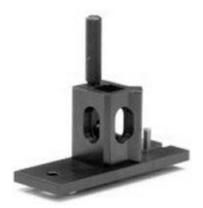
**Figure 1.** The single sample holder, note the lever on the top for easy lifting of cells. This lever can also be used to alter the height or the cuvettes.
