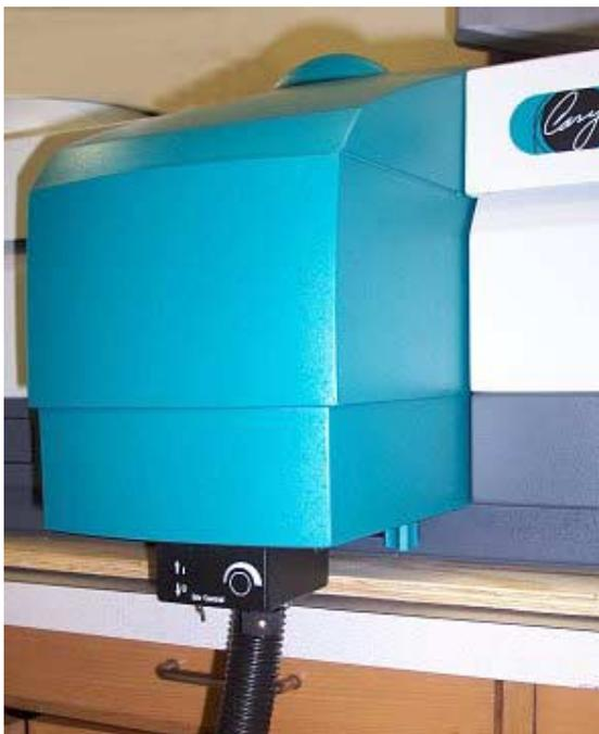
The extended sample compartment fitted with a multicell holder.
