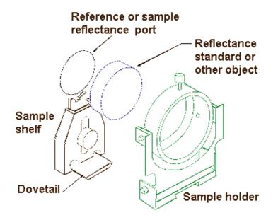
Figure 48. The sample is mounted at the reflectance or reference port using the sample holder.
