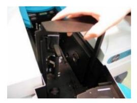
Figure 47. Removing the light seal.
