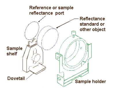
*Figure 24. The sample holder fits onto the dovetail at either the reference or reflectance port.*
