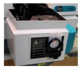
Figure 26. Checking the beam at the reflectance port.
