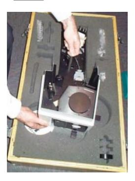
**Figure 18.** Lift the DRA from the wooden packing case as shown. One hand on the "T" handle, the other under the corner marked "Lift here".
