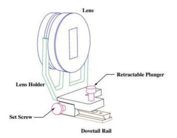
Figure 34: The small spot kit lens holder, rail and lens.
