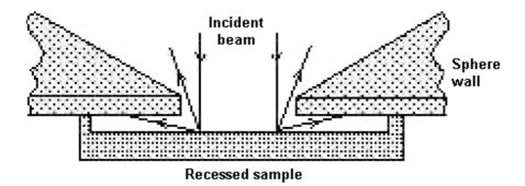
*Figure 5:* Some of the wide-angle scatter is lost when there is a space between the sample and the sphere wall
