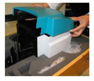
Figure 16. Removing the accessory cover.
