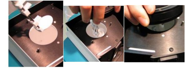
Figure 30. Lower the centre mount through the opening in the sphere, user the locating holes in the top of the sphere to secure the centre mount.
