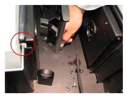
Figure 23. Place the front lock down pin into position.
