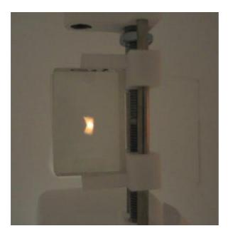
Figure 52. The small spot kit beam falling on a sample using one of the centre mount options.
