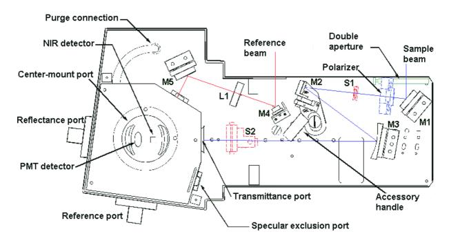
Figure 9: A schematic view of the external DRA.
