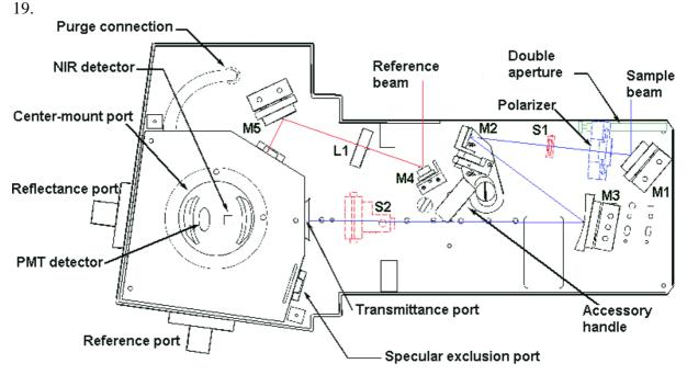
*Figure 19:* The Varian 900, 1800, 2500 Diffuse Reflectance accessory with the optics cover removed. The large reference plate is clamped over the sample port at the centre of the sphere cap.
