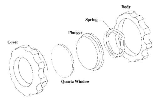
Figure 40. An exploded view of the powder cell.
