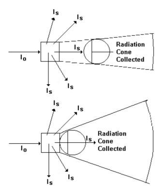
*Figure 4:* Collection of scattered light by an integrating sphere.  $I_o$  = incident light,  $I_s$  = scattered light.
