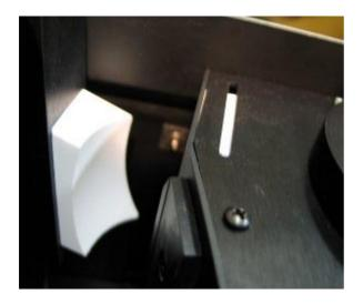
Figure 20. Install the specular port plug.
