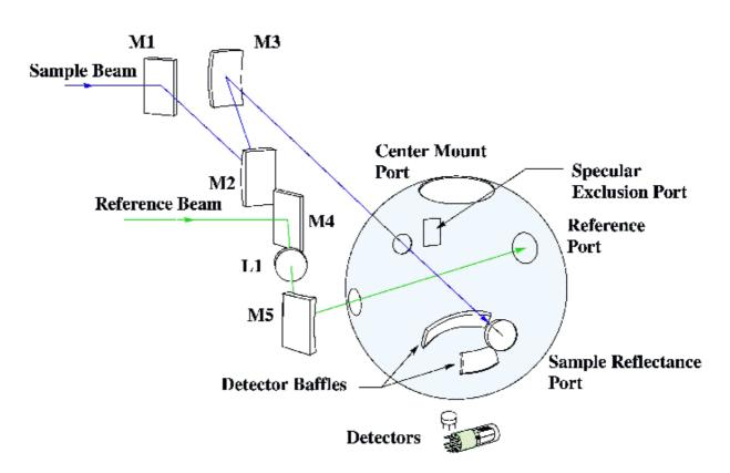
Figure 10: The optical design of the external DRA.
