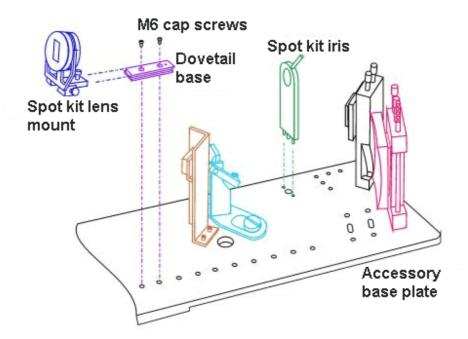
Figure 35: Installing the small spot kit.
