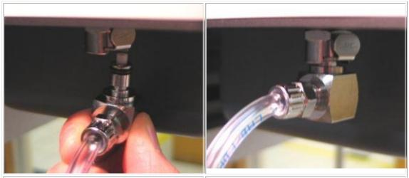
**Figure 54.** Attach the connector on the hose to the connector on the under side of the integrating sphere. **Figure 55.** The connectors snap together.
