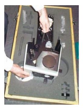
**Figure 21.** Lift the DRA from the wooden packing case as shown. One hand on the "T" handle, the other under the corner marked "Lift here".
