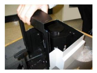
Figure 17. Removing the light seal.
