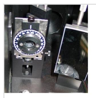
Figure 45. The polarizer attachment in the DRA.
