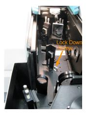
9. Take care to align the metal edges of the DRA with the guide tabs on the edge of the instrument sample compartment. This will correctly align and engage the rear lockdown pins into the sample compartment floor. See photos to see how to line up the tabs, note in particular the red circle indicating where the tabs should sit.
