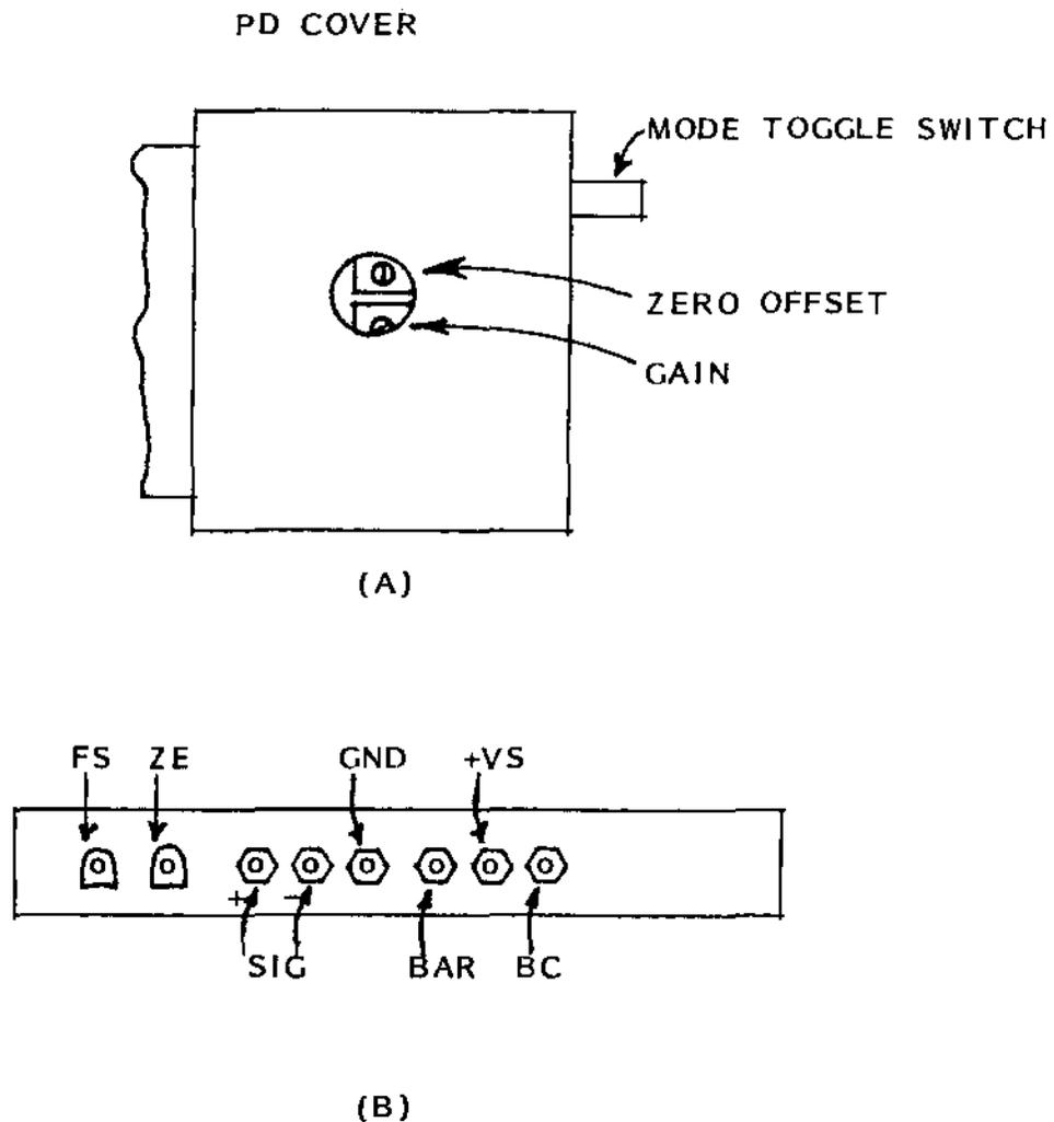
**Figure 7-5.** The upper diagram ( A ) shows the photodetector circuit board in the analyzer module. The lower diagram ( B ) shows the two trimpots ( FS and ZE ) and the six voltage test points at the rear of the LED meter.
