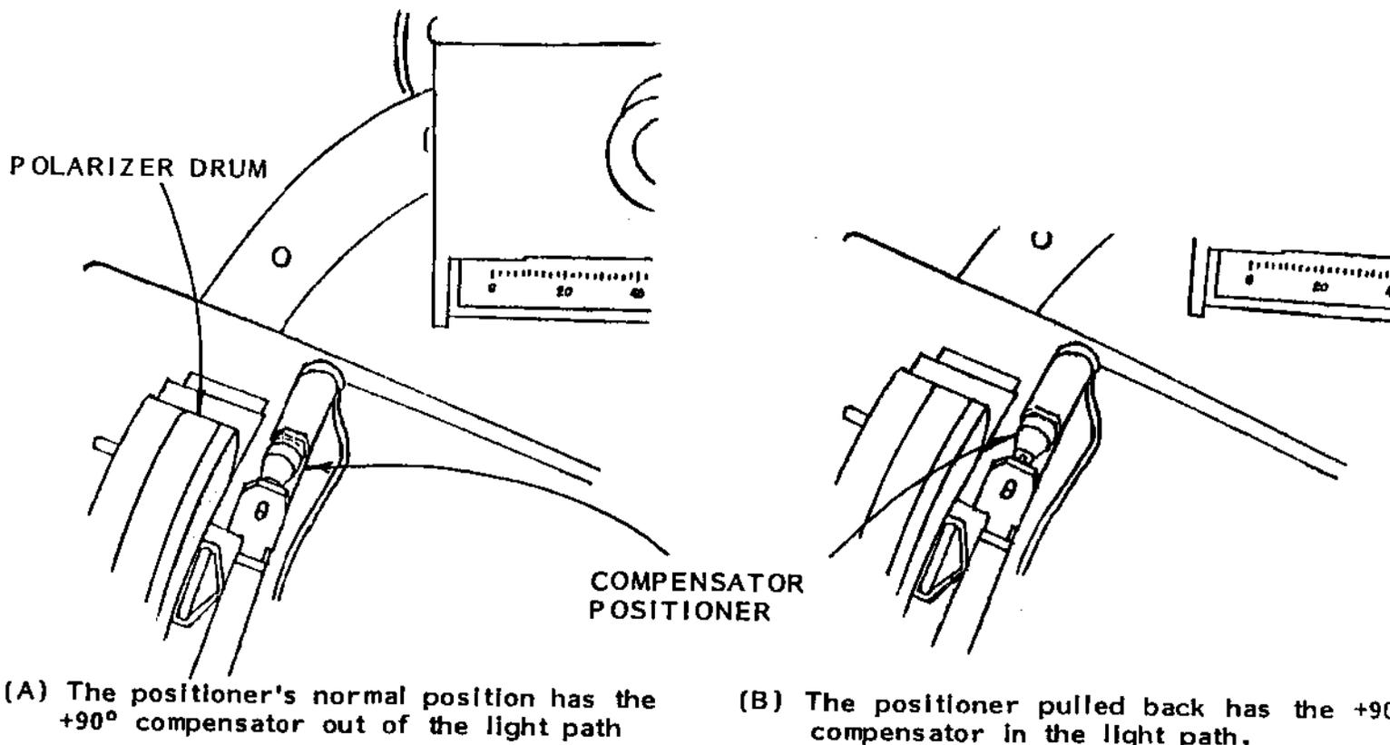
Figure 7-7. This is the automatic compensator positioner on the right end of the polarizer arm.
