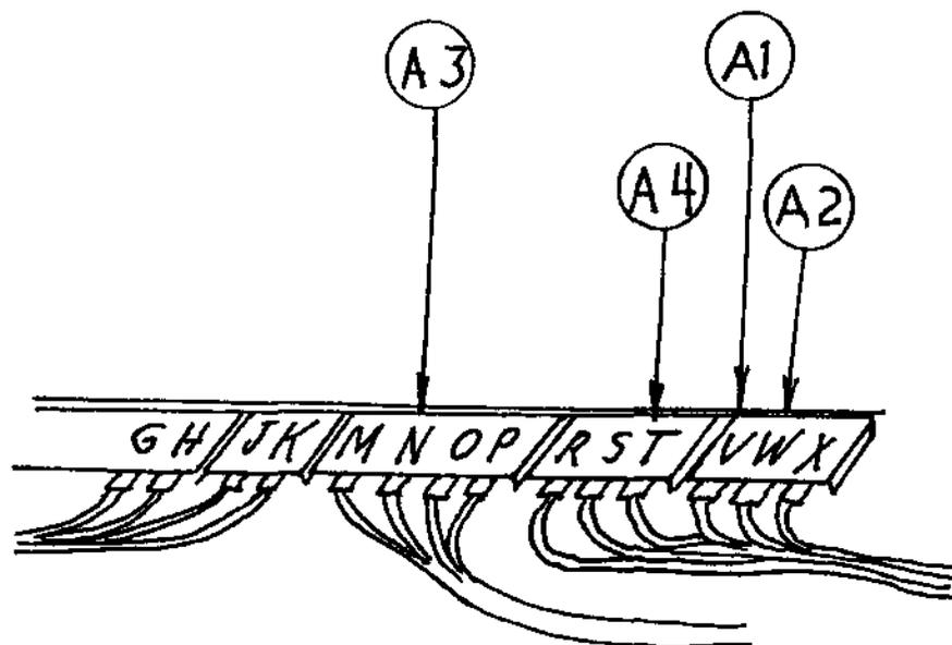
Figure 7-4. These are the four Check Points ( A1 to A4 ) in Figure 7-1 ( which does not show A2 ). In order to observe the waveform or measure the voltage, carefully pull out the appropriate connector just enough to carefully insert a sharp probe ( with the common probe at the black test jack ).
