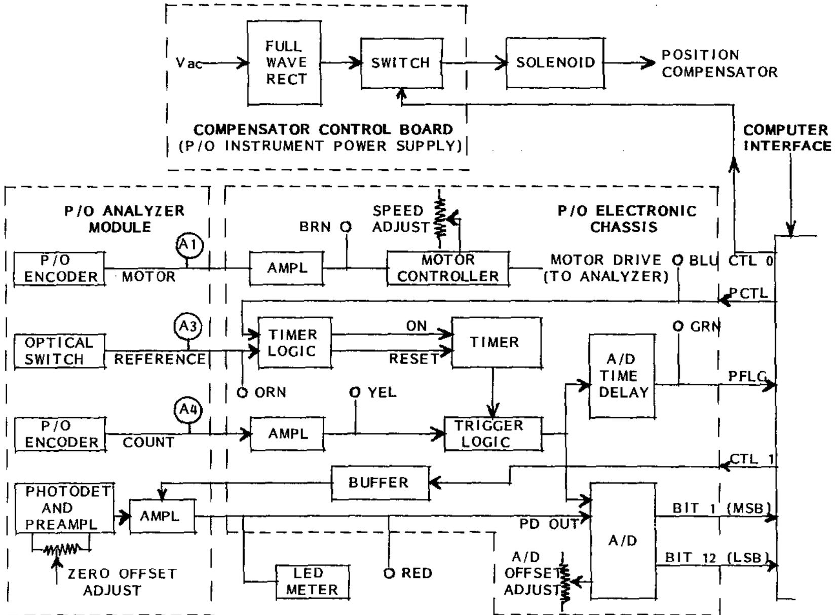
Figure 7-1. This is the Measurement System Functional Diagram.
