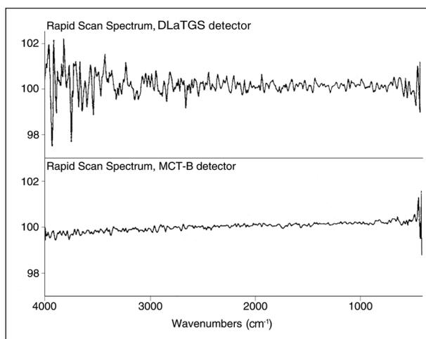
Figure 2: Rapid-scan data comparison of MCT-B to DLaTGS detectors
