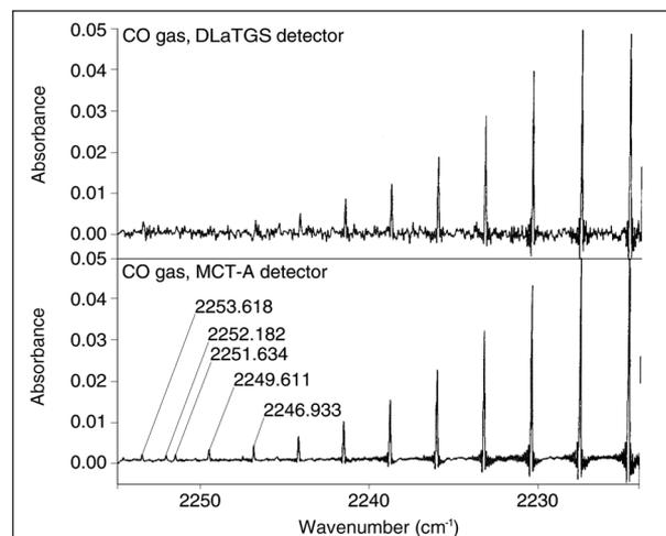
Figure 1: High-resolution gas analysis comparison of MCT-A to DLaTGS detectors
