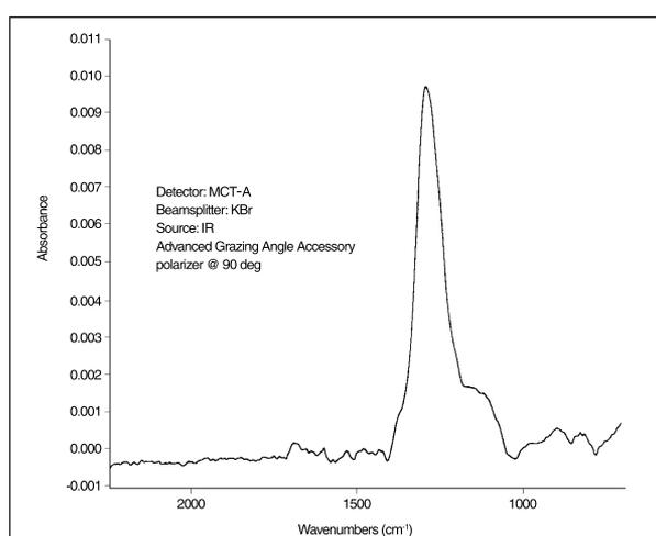
Figure 3: Grazing-angle spectrum of a 40-angstrom thick lubricant
