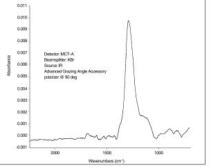
Figure 3: Grazing-angle spectrum of a 40-angstrom thick lubricant
