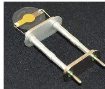
8. Assemble the eQCM cell with your crystal and connect to the 10M fig 2.
