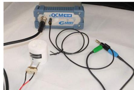
Figure 2 eQCM cell with electrical Connection to 10M
