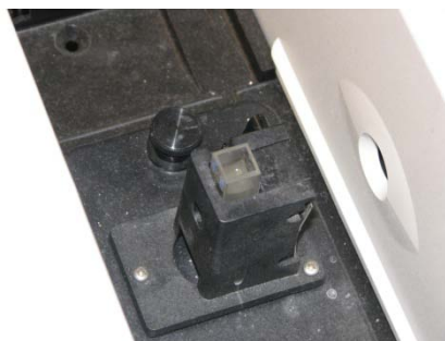
Cuvette mounted in the sample holder
