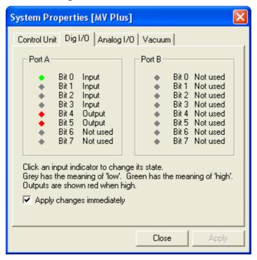
If the control unit that you have created has available digital I/O, you will have a digital I/O tab which will show the state of the 16 digital I/O lines. Once again the exact content of this page depends on how the control unit is configured. Hardware set-up can of course be used to change the I/O configuration, or it can be set when the virtual instrument is created, using the Options... button.
