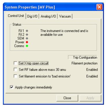
The first tab of the system properties window is a simulation of the standard control unit itself. You will notice it has the same LED's as a Microvision Plus/HPQ, which function in exactly the same way as a real control unit. If the control panel is running but the RGAServer is not, the comms light will be slowly blinking. If the server is running the comms light will be solid green.
