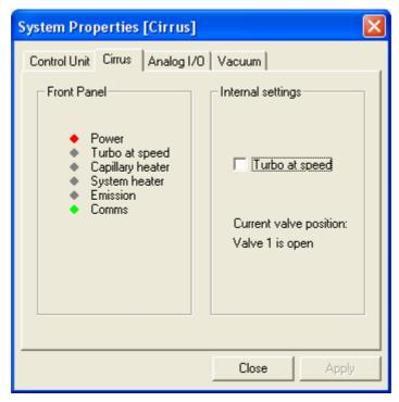
If the virtual system is a Cirrus, you will have a Cirrus tab. This shows the same LED's that are found on the front of the real Cirrus hardware. The only interactive 'input' that is available is the 'turbo at speed' setting. The behaviour of the filaments mirrors the real system. Filaments can only be on when the turbo is at speed and the system pressure is less than 5e-5 mbar.
