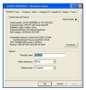
The General tab displays many fixed items of information, including the embedded software versions. The three user-configurable settings are the name assigned to the control unit, the mains frequency and the filament type. You may also use this page as another way to download new embedded software to the control unit.
