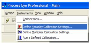
To define the calibration, select **Define Faraday Calibration Settings** from the **Instruments** pull down menu.
