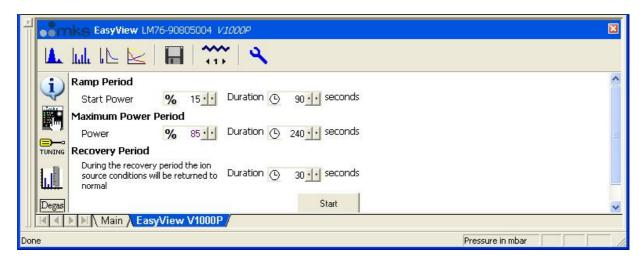
When EasyView degasses an ion source it ramps up to full power over a user defined period of time. It then maintains that power for a further period. When degas is complete it resets the ion source conditions to 'normal' and waits for a period of time during which the temperature of the source can stabilize.
