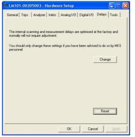
This tab is an advanced feature. The control unit has a table of software delays that control the length of transition states – for example how long to wait when switching between a Faraday and multiplier detector.
