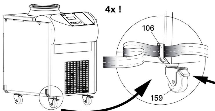
**Fig. 5: Anchoring the pumping station**
