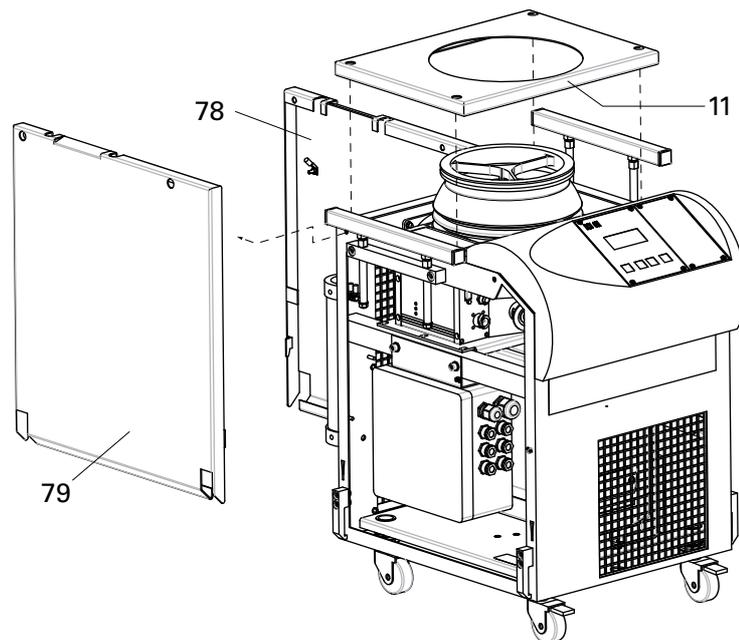
**Fig. 9: HiCube Classic, dismantling the casing panels**
