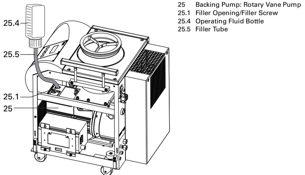
**Fig. 8: Filling the backing pump with operating fluid**
