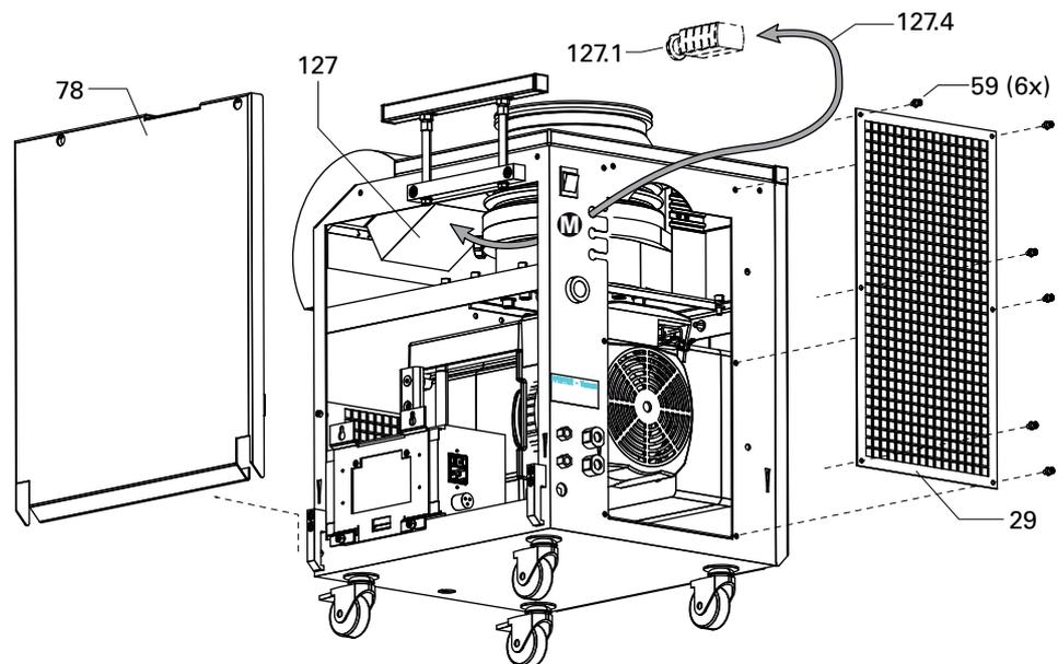
**Fig. 6: HiCube Classic, Running a measuring cable**
