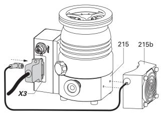
215 Pump lower part215b Air cooling unitX3 Multi-functional connection
