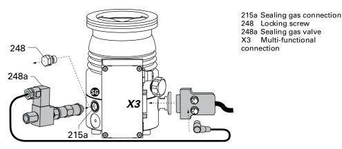
Fig. 12: Connecting the sealing gas valve
