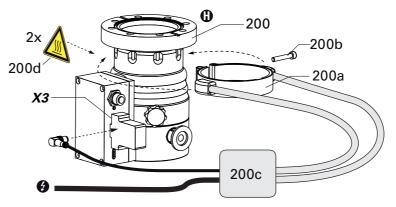
Fig. 10: Connecting the heating jacket
