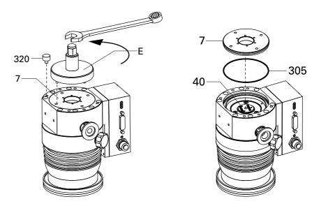
Fig. 15: Assembly / Disassembly of the operating fluid reservoir
