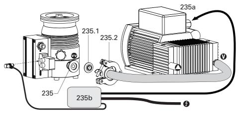
Fig. 7: Connecting the backing pump
