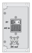
S1 Switch ON/OFF AC in Mains connection DC out Connection TC 110
