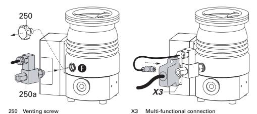
Fig. 9: Connecting the venting valve
