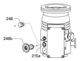
215a Sealing gas connection248 Locking screw248a Sealing gas throttle
