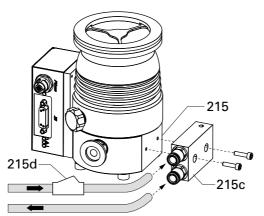
215 Pump lower part,215c Water cooling unit215d Dirt trap
