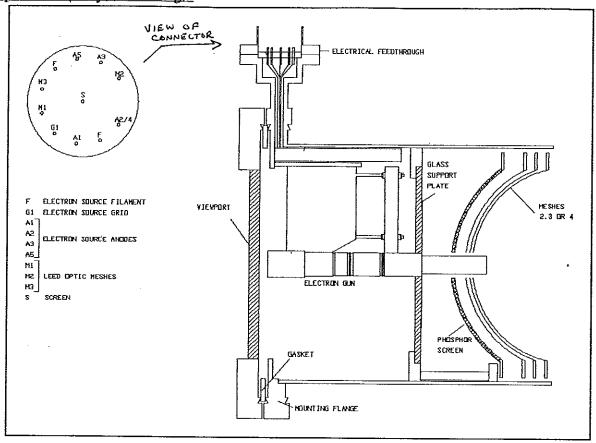
A general view of the Rear View LEED optics is shown. The optics assembly is mounted on a single 200mm conflat double-sided flange and includes two main components: the electron gun and mesh assembly. Four long rods attached to the mounting flange provide support for the whole assembly. Bolted to the end of the four rods is a mounting ring, which holds a flat glass plate. The mesh assembly is supported from the mounting ring by means of three shorter rods.
