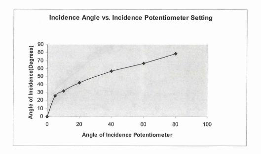
Figure 6. Showing the required setting for the rear panel Y- Incidence Angle Correction potentiometer in order to compensate for an oblique geometry.
