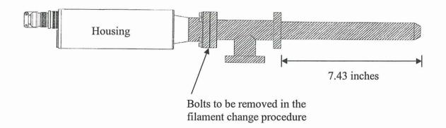
Figure 3. Ion Gun Schematic.
