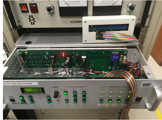
Figure 2 X-ray gun power supply with cover open and spot size control box sitting on top
