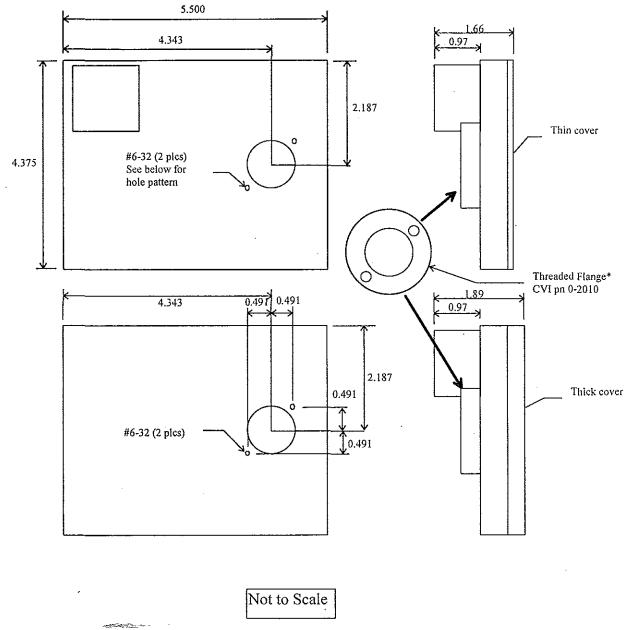
\* Threaded flange is Thorlabs 1" tube compatible.
