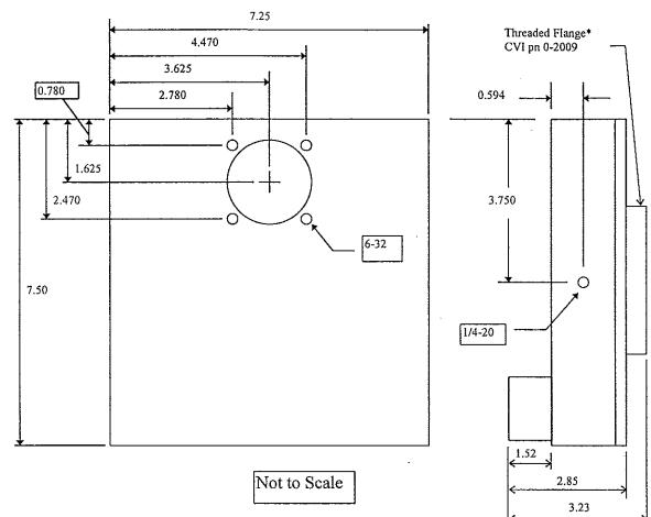
\* Threaded flange is Thorlabs 2" tube compatible.
