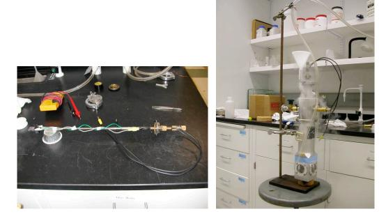
7. Mount the base in the CARY and set up using the saved "stark\_method". Place dewar in CARY (black material) and go to Align to turn on white light (don't press OK). Check with paper. Determine plate spacing from the interference pattern
