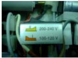
1-phase, 100V power source
