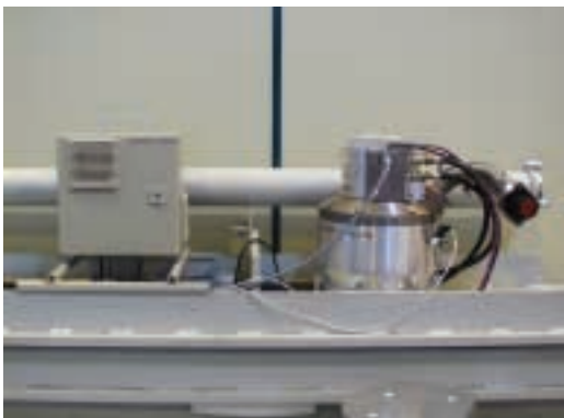
Glass coating system with 22 TPH 2101 UP. The electrical cabinet (protection class IP 54) contains all electrical components to operate the pumps. All functions of the pumps are controlled via profibus. Saint Gobain Glass, France
