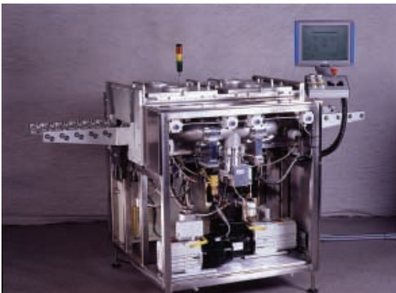
Semi automated Wafer Bonding System. Fully automated cassette-to-cassette align and bond operations for MicroElectroMechanicalSystems and Silicon-On-Isolator production. Advanced spray coating technology. Turbo Drag Pump TMH 071 P and Diaphragm pump. EVGroup, Austria
