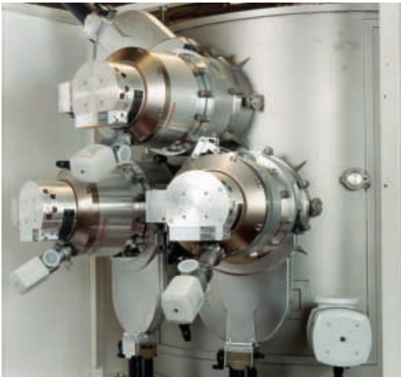
Ophthalmic Coaters. Deposition of anti-reflection films on lenses. CompactTurbo TPH 2101, Rotary Vane Pump DUO 65 and Valves EVB 100, EVB 040. Satis, Italy
