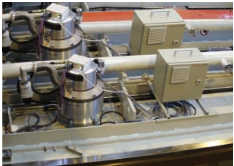
Glass coating system with 22 TPH 2101 UP. The electrical cabinet (protection class IP 54) contains all electrical components to operate the pumps. All functions of the pumps are controlled via profibus. Saint Gobain Glass, France
