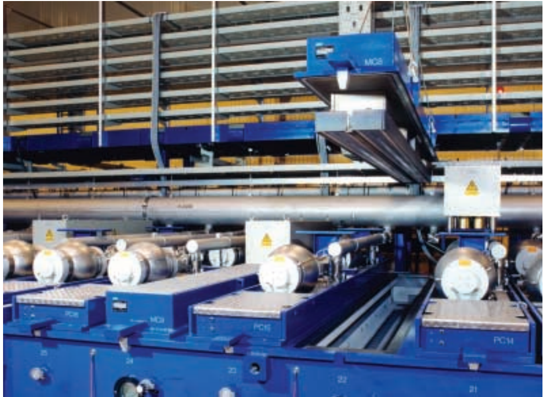
Glass coating system. Coating architectural glass with 15 CompactTurbo 2201. Von Ardenne Anlagentechnik, Dresden, Germany
