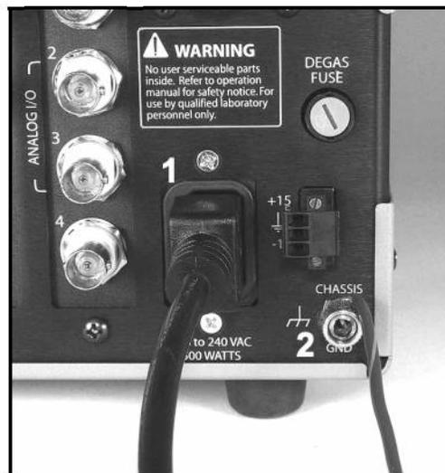
Figure 1-2. Power and chassis-ground connection on the back of the IGC100 controller.
