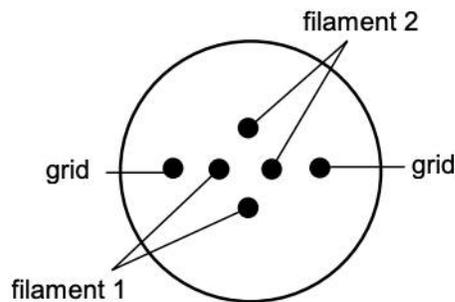
*Figure 1-12. Pin alignment for base connector of a glass-tubulated gauge w/dual filament.
