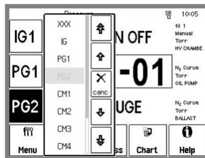
Figure 1-35. Select CM1 for the lower Data Bar.
