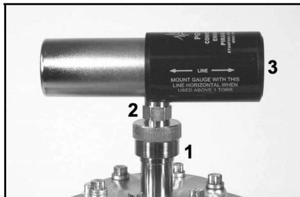
*Figure 1-22. PG105 gauge mounted on a 1/2" compression fitting in the horizontal mounting orientation required for pressure readings above 1 Torr. 1. Ultra-Torr<sup>®</sup> fitting, 2. Side port tube (OD 1/2") with built-in nut, 3. PG105 Body.*
