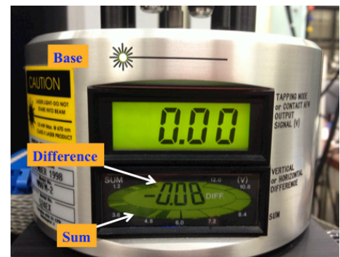
Figure 5. The sum and difference values on the lower display. The sum is shown by the hash marks around the edge and must be maximized. The difference should be minimized
