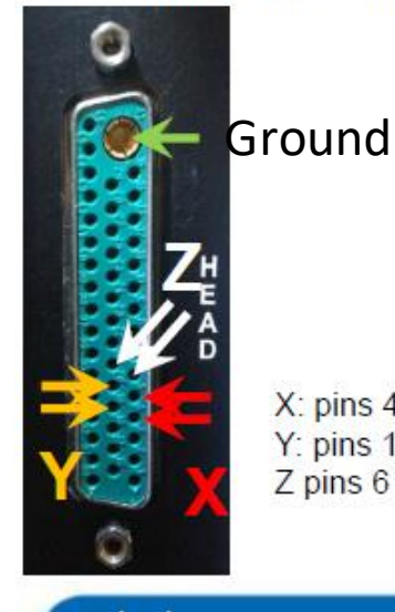
Figure 15. Pin layout of the scanner connector
