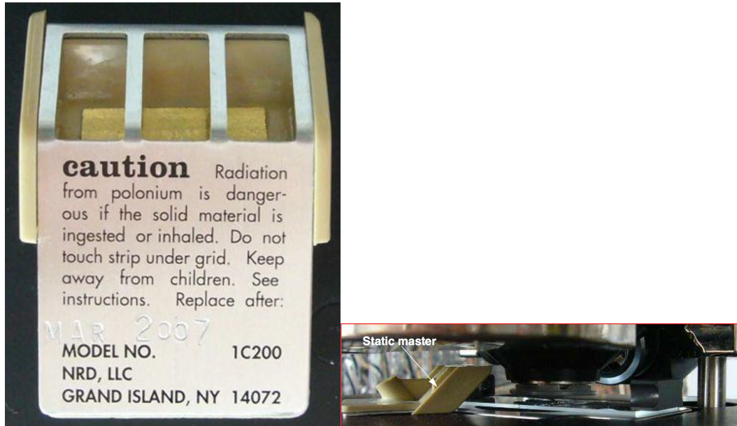
Figure 4.5.: Placing static master near sample on an MFP-3D AFM to dissipate charge.
