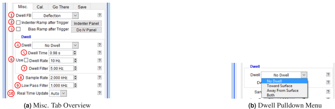
Figure 18.6.: The Misc. Tab allows the user to define temporal and low pass filter settings for dwell and force curve collection.
