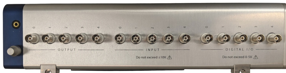
Figure 16.2.: Side view of Backpack Controller showing BNC connections.
