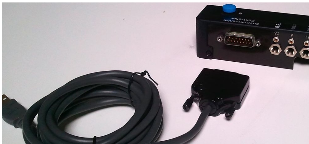
Figure 33.18.: Cable 448.130 supplies 5V to the junction box leak detection circuit. Plug one end into a free USB port on your PC, the other end into the junction box as shown.
