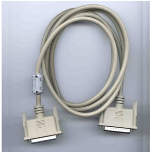
(a) 448.023 cable, DB25, modified with interrupted outer shield.
