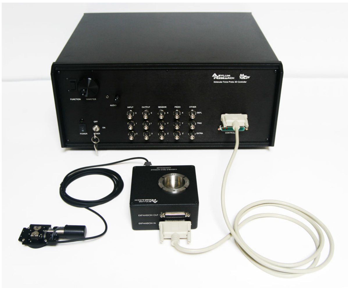
Figure 32.2.: The VFM sample stage plugs into the 9-pin connector on the VFM controller box. This in turn plugs into the 25-pin expansion connector on the front of the MFP-3D controller. This photo shows the older MFP-3D controller. The newer ARC2 controller can be used as well.
