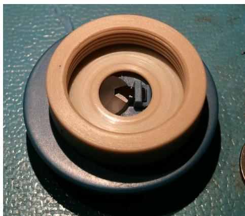
(a) Cantilever holder clearance when using the thin film sample mount. Note that for optimal clearance the cantilever does not land in the center of the visible part of the sample.
