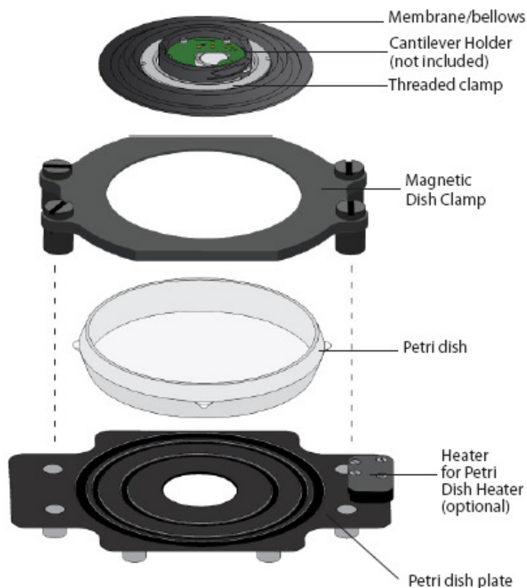
Figure 26.2.: Schematic diagram of complete assembly, in this particular case with the Petri Dish Heater stage.
