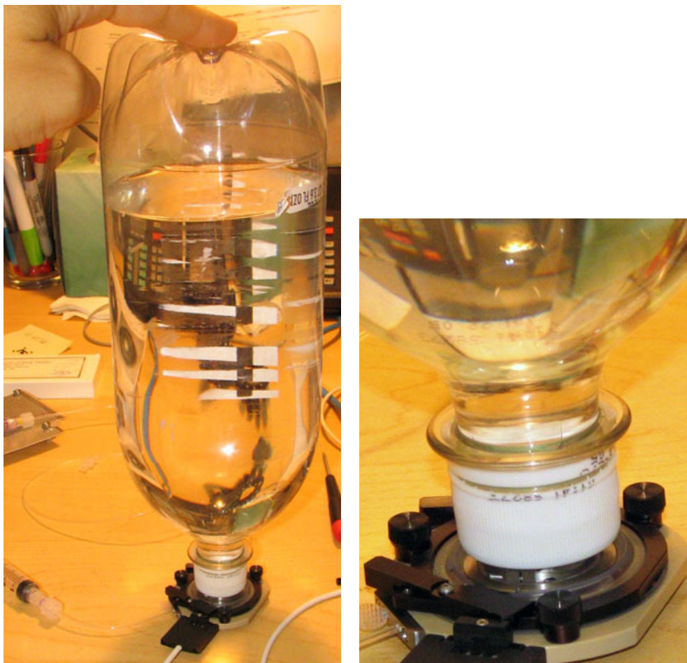
Figure 22.6.: Maximum pressure test by placing a weight onto a fully sealed closed fluid cell. Note the picture shows the Bioheater variation of the Closed Fluid Cell. Observe that the jaws on the clamp are OPEN to perform this test. Otherwise the clamp would support the weight of the bottle, and not the fluid inside.
