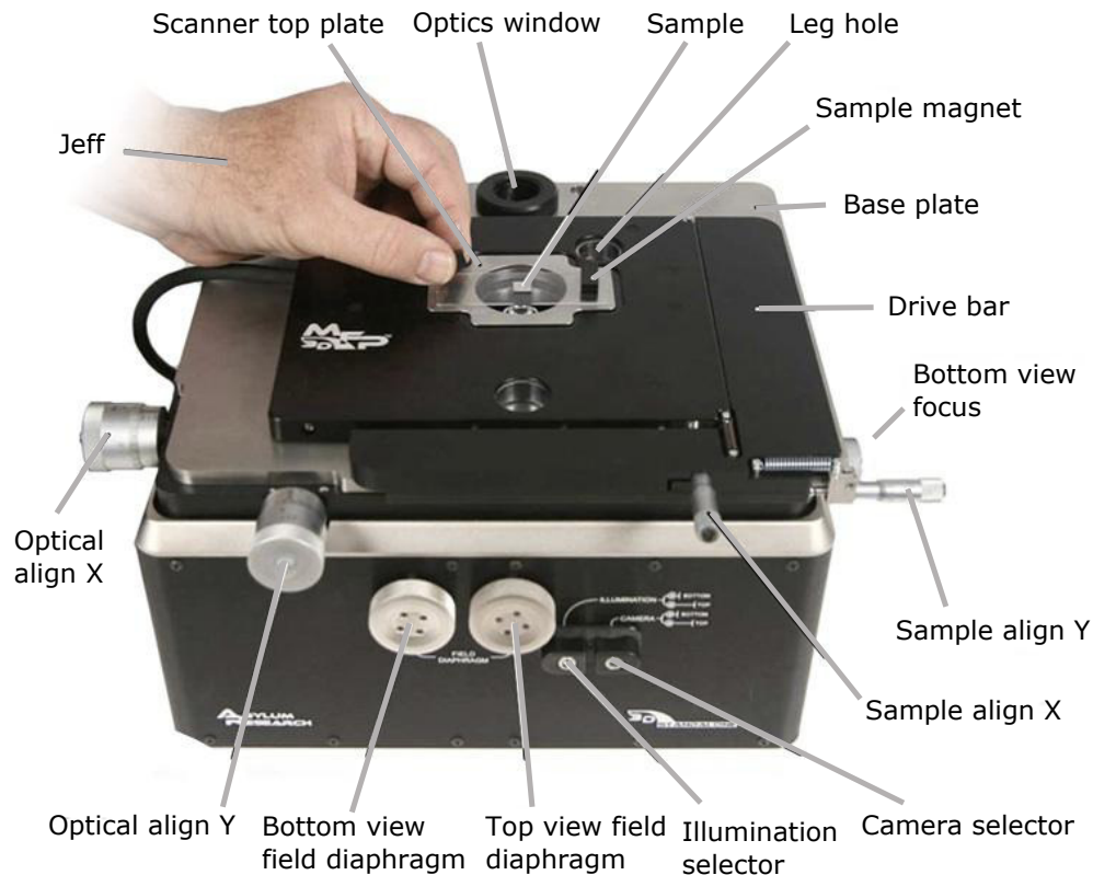
Figure 1.5.: Controls on the SA Base. Missing from view are (on the left) the aperture diaphragm which is a knurled ring around the entry point of the fiber optic illumination and (on the right) a large knob for focusing the bottom view objective.
