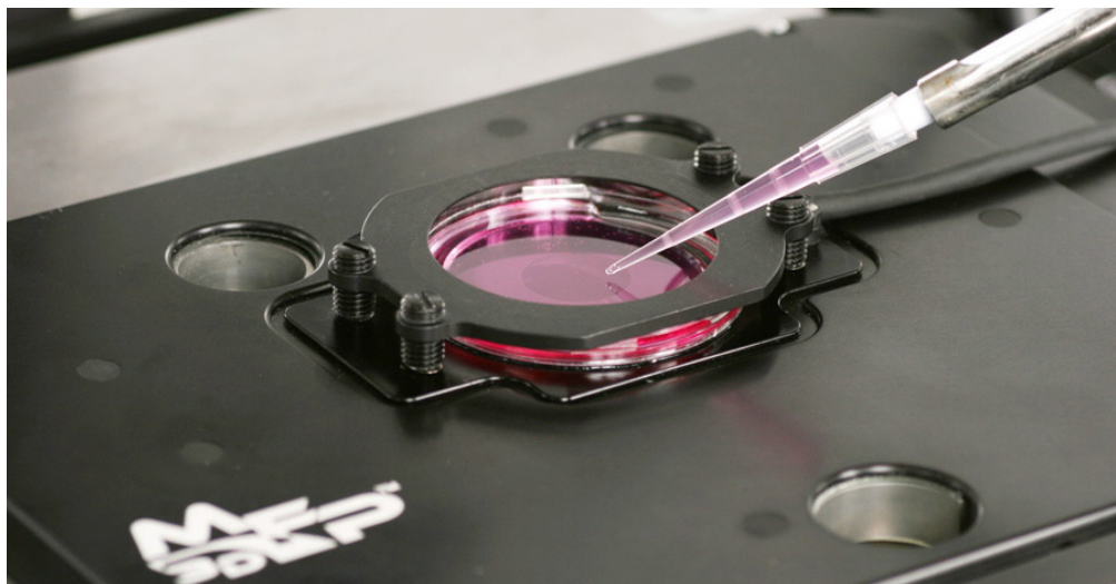
Figure 27.5.: Picture of Petri dish with clamp sitting on the scanner. Open access to the sample when the head has been removed.
