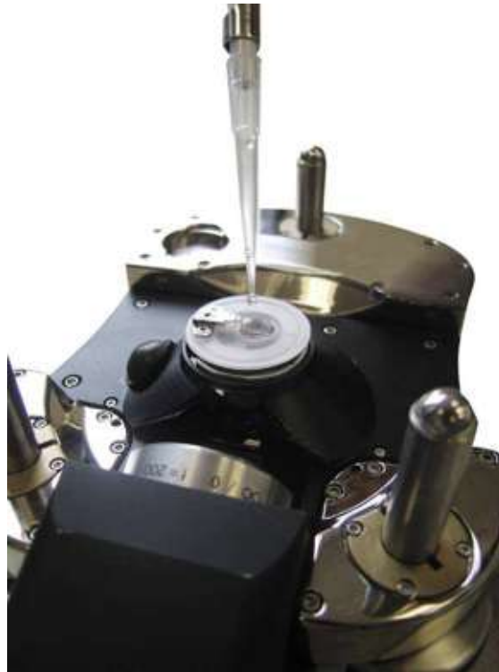
Figure 8.3 Close view of how to pre-wet the cantilever with a pipet before immersing it in liquid
