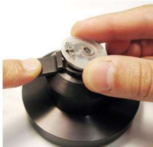
Figure 5.12 Prepare the Cantilever Holder. Figure A Remove from Head. Figure B Place in Holder
