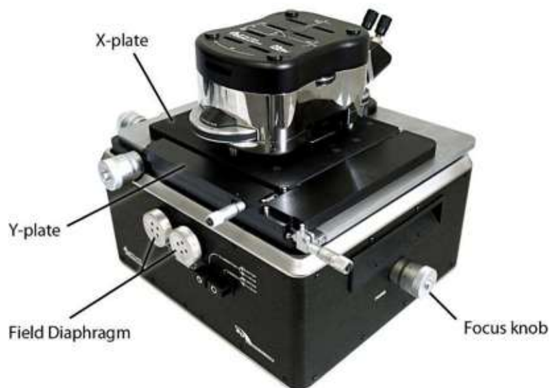
Figure 5.21 Bottom View Camera X and Y Position
