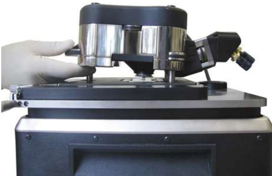
Figure 8.19 This side view shows how to lift the MFP-3D™ head to straighten bent cantilevers or tap it to remove air bubbles. This procedure can also be used to eliminate bubbles stuck on the cantilever: tap the front leg a few times on the stage and check optically for the bubbles.
