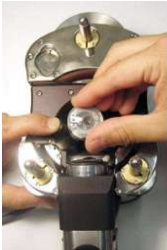
Figure 5.12 Prepare the Cantilever Holder. Figure A Remove from Head. Figure B Place in Holder
