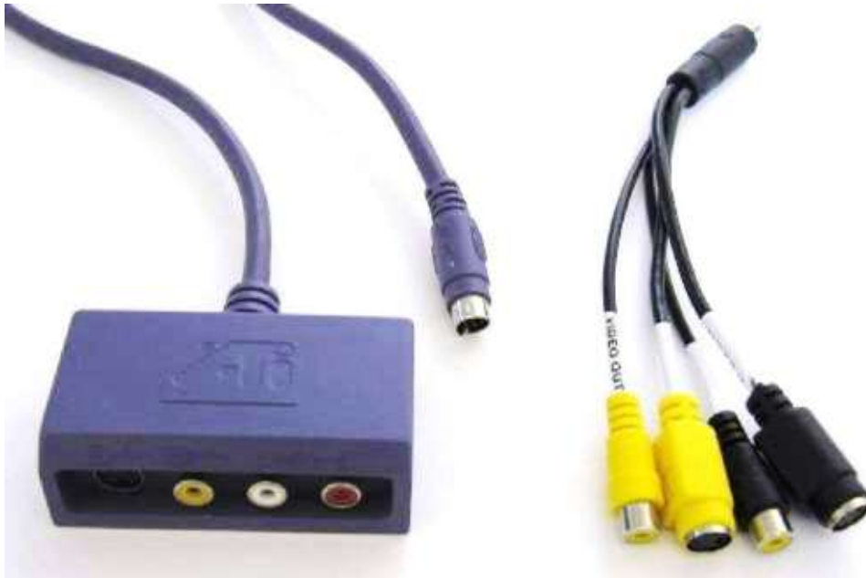
Figure 5.41 Video Port Connections. The older “Barney” version is shown on the left and the new connectors on the right
