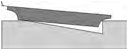
Bad Cantilever Position
