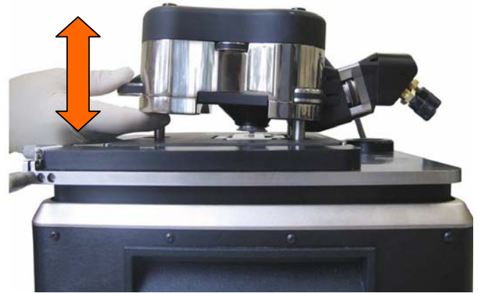
Figure 6.2.2: Lift head in and out of the fluid on sample to remove air bubbles.
