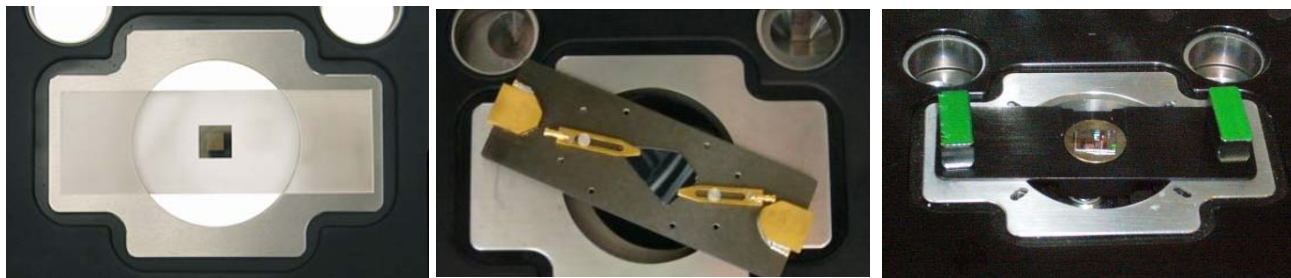
Figure 3.2.2: A) Place sample area of interest towards center of scan plate; B,C) multiple sample holders can be magnetically held down on the MFP3D.
