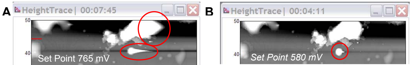
Figure 6.1.8: Increasing Set Point force (i.e., lower set point voltage) to improve tracking over large surface asperities: A) before adjustment- 'Gentle' engage Set Point force (i.e., lowest set point force to engage); B) increased Set Point force increases cantilever dampening to reduce poor tracking
