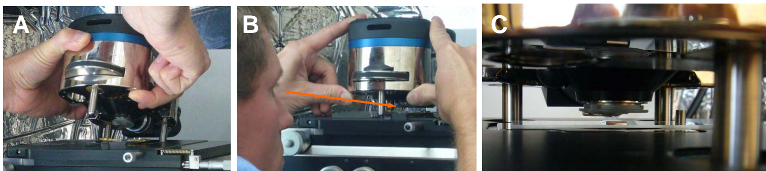
Figure 3.3.1: Placing head on sample stage: A) place back legs into kinematic ball joints ; B) look at tip sample distance as front of head is lowered down, always ready to pull head up if tip appears to get too close (<1mm) ; C) space between tip and sample should be visible when all three legs are on stage baseplate.
