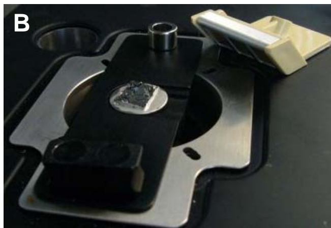
Figure 9.3: trying to eliminate charge by removing any glass components in sample mounting. Here, the sample (graphite) is fixed to sample puck via silver paint, and placed on an AR magnetic sample holder.
