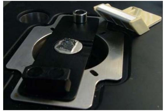
Figure 6.1.14: eliminating charge by removing any glass components in sample mounting. Here, the sample (graphite) is fixed to sample puck via silver paint, and placed on an AR magnetic sample holder.
