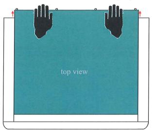
cover and press with your fingers on the rear panel, while pressing on the top cover. Now the top cover will slide off easily.
