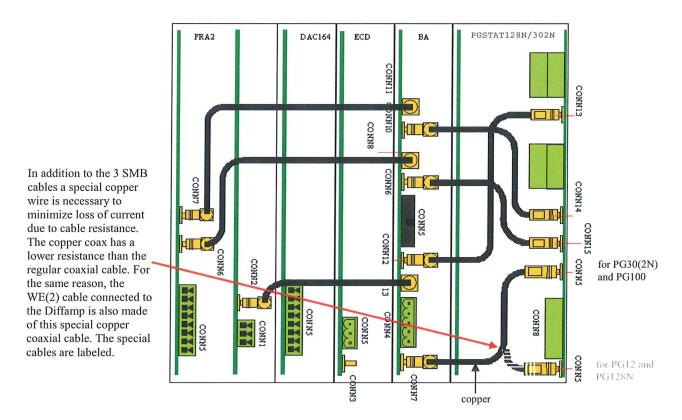
Note: The supplied jumper cable is NOT used for the BA module in an 8-series instrument!
