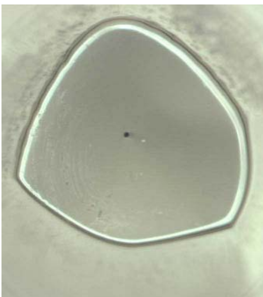
Figure 3: Smoothly polished 25 \mu\text{m} Pt UME that has been slightly sharpened.
