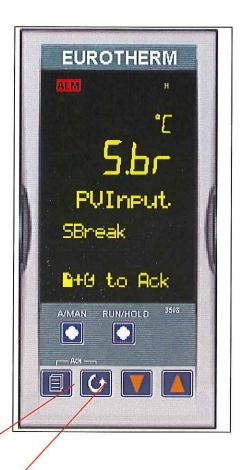
Press the picture- an parameter key together to reset the alarm.
