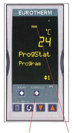
At automatic mode press 2x the RUN/HOLD key until Run appears at the display. The program is running.
