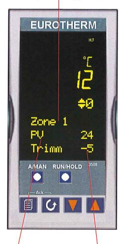
The actual temperature (PV) and the trimm (Trimm) from the zone appears.
