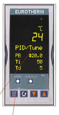
Go to PID/Tune screen via picture key. Here you can modify the control parameters via the plus / minus key.
