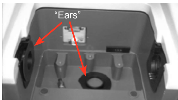
Figure 3 The accessory compartment showing “ears”.
