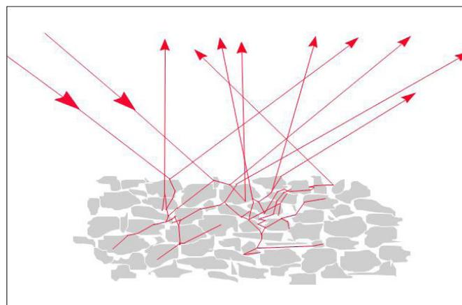
Figure 4. Diffuse reflection by a powder
