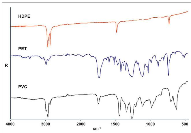
Figure 13. Spectra of soft drink bottles on silicon carbide abrasive.
