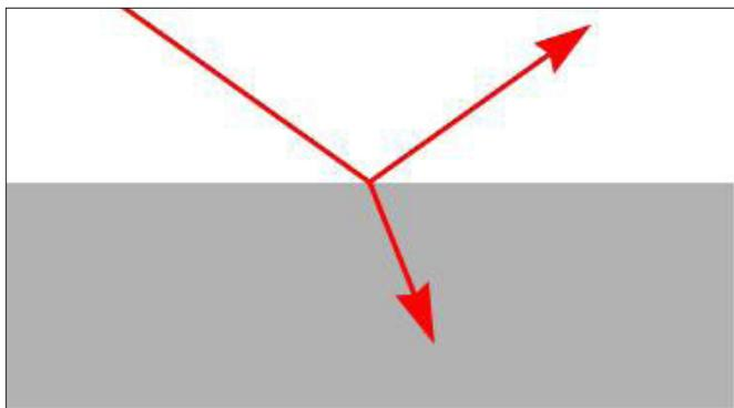
Figure 1. Reflection and transmission at a plane surface
