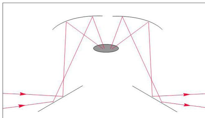
Figure 12. Optical arrangement for diffuse reflection.
