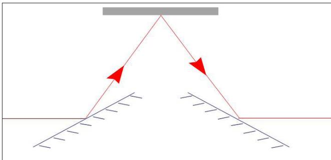
Figure 9. Optical arrangement for measuring specular reflection.
