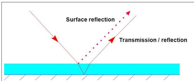
Figure 10. Transmission/reflection through a coating.
