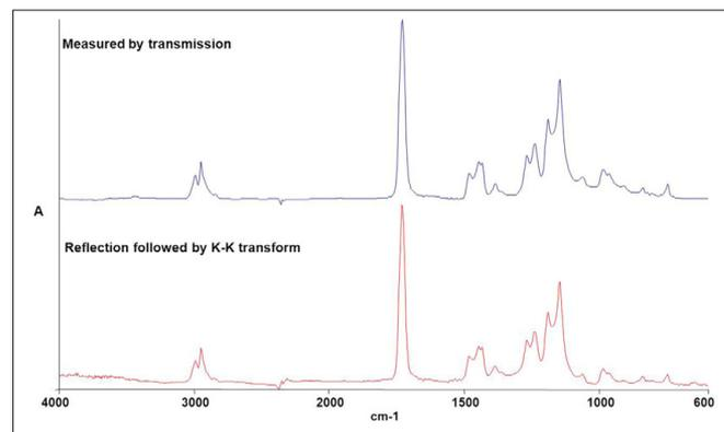
Figure 3. Transmission and Kramers-Kronig transformation of the reflection spectrum of polymethylmethacrylate
