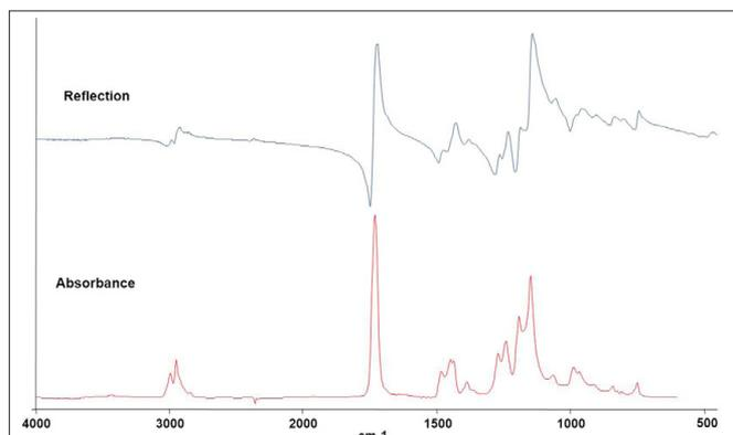
Figure 2. Reflection and transmission spectra of polymethylmethacrylate
