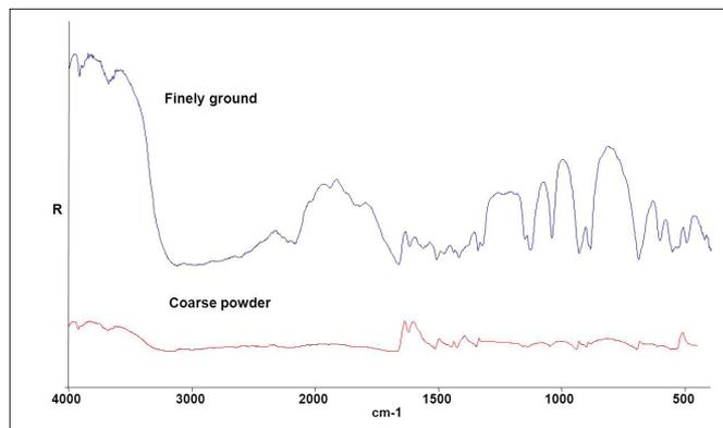
Figure 5. Diffuse reflection spectra of glycine (the upper one is offset for clarity).
