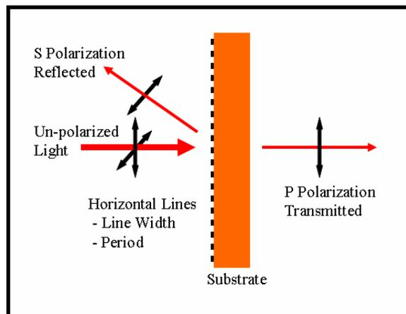
The overall transmission characteristic of the polarizer depends upon the substrate, but the polarization
