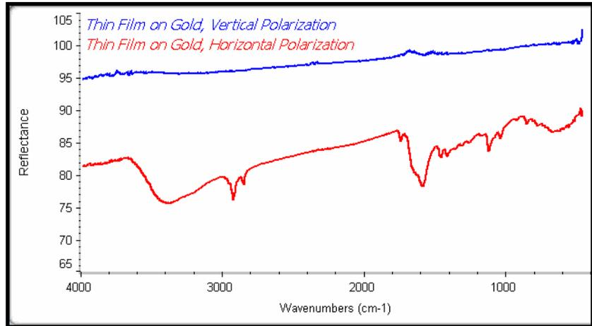
metallic mirror surface is enhanced. The spectrum measured with the polarization perpendicular to the surface (electric vector parallel with the surface) is not detected. The non-polarized light measurement is a combination of the two polarized
