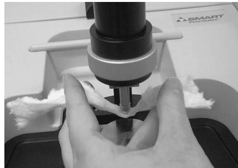
Figure 9: Removing sample from the tip of the pressure applicator.
