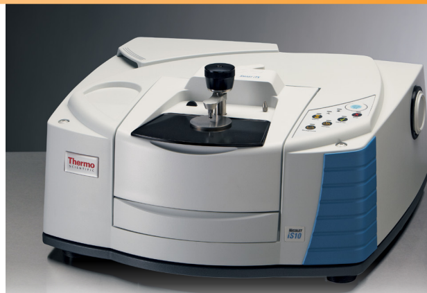
Figure 1: Thermo Scientific™ Nicolet™ iS™10 FT-IR spectrometer with Smart iTX accessory
