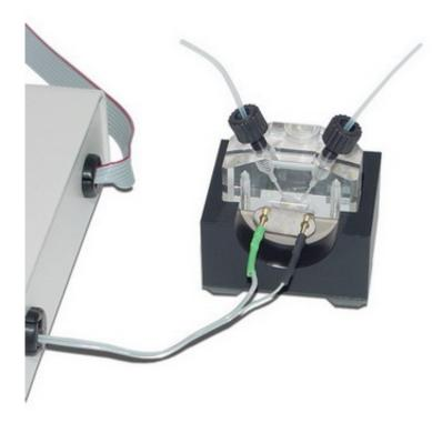
The Resonance frequency of quartz changes when material attaches to the electrode's surface. This product is capable of super-micro quantitative analysis by using this unique behavior.
