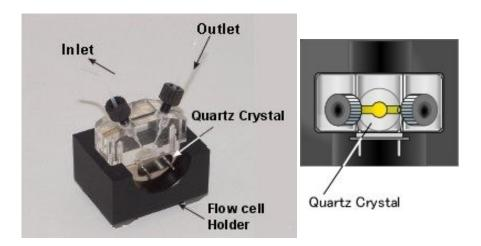
**EQCM Mode** Using electrochemical absorption
