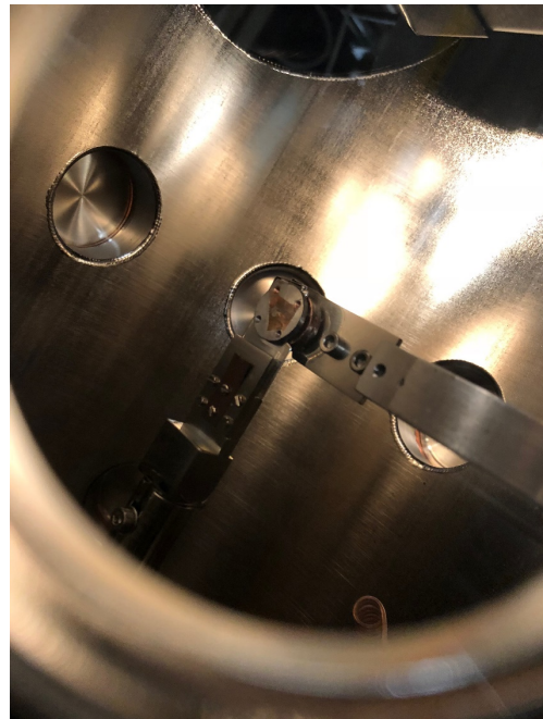
Figure 5 View into STC with transport arm extended into the chamber and transferring puck to STC to SAC arm.
