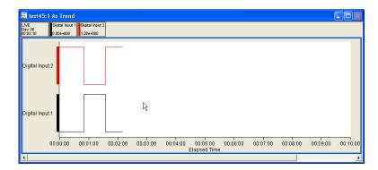
This option is only useful for displaying digital data. In the above example, there are two digital input channels with both channels configured to "draw stepped".
