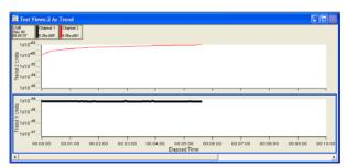
This is a 2-pane trend with channel 1 displayed on trend pane 1, with its own measurement units, and channel 2 displayed on trend pane 2 with different measurement units.
