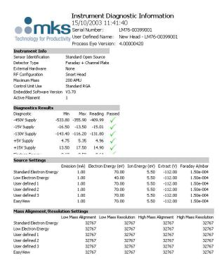
The report contains information about the control unit configuration, ion-source settings and mass alignment/resolution settings as well as power supply levels.
