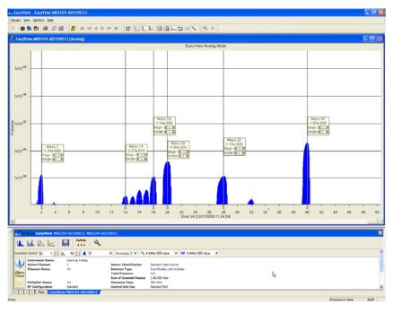
While in the mass tuning mode mass alignment flags are placed on screen. The vertical position of these flags can be adjusted if needed.
