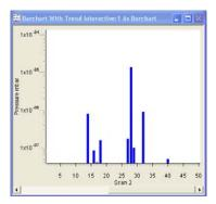
"Swept Measurement" view, this is a display of partial pressure versus mass. Bar chart shown below, where there is a single bar shown per mass.
