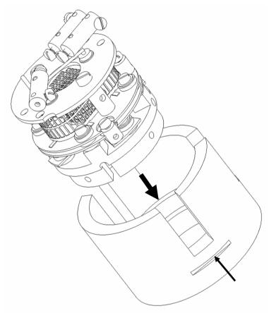
Note the orientation of the source assembly when inserted into the jig. Align the extract plate's barrel connector with the alignment indicator on the jig.
